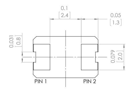
Note: Due to availability of the ceramic base, a chamfer may appear on pin 1.
