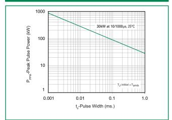
Figure 3 - Peak Pulse Power Derating Curve
