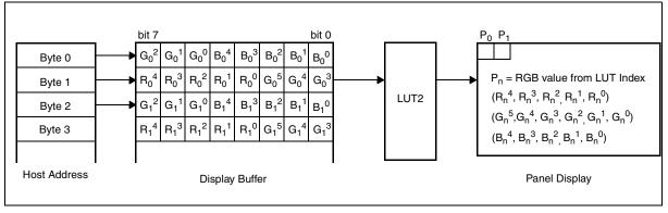
Figure 13-4: LUT2 for 16 Bpp Mode
