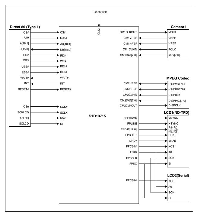
Figure 3-2: S1D13715 System Diagram 2
