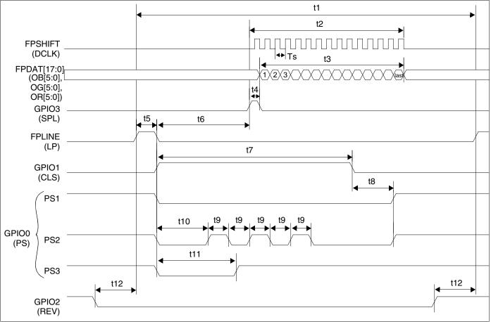
Figure 7-33: HR-TFT Panel Horizontal Timing
