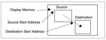
Figure 16-2: Move BitBLT data flow
