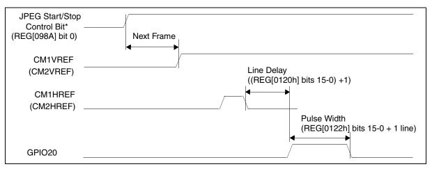
Figure 20-1: Strobe Signal Output Timing
