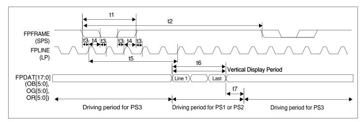
Figure 7-34: HR-TFT Panel Vertical Timing
