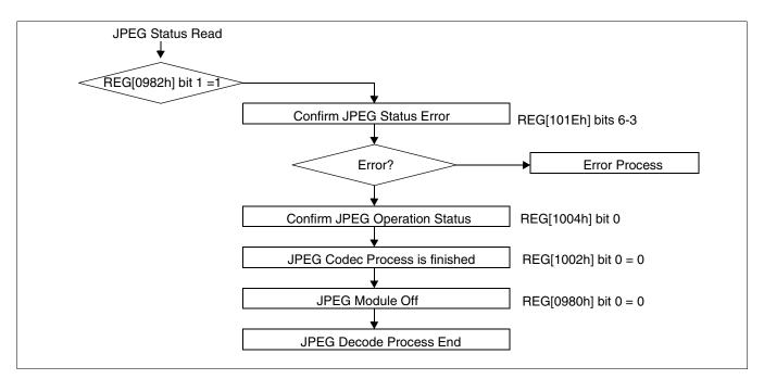
Figure 19-19: JPEG Decoding Process (6 of 6)
