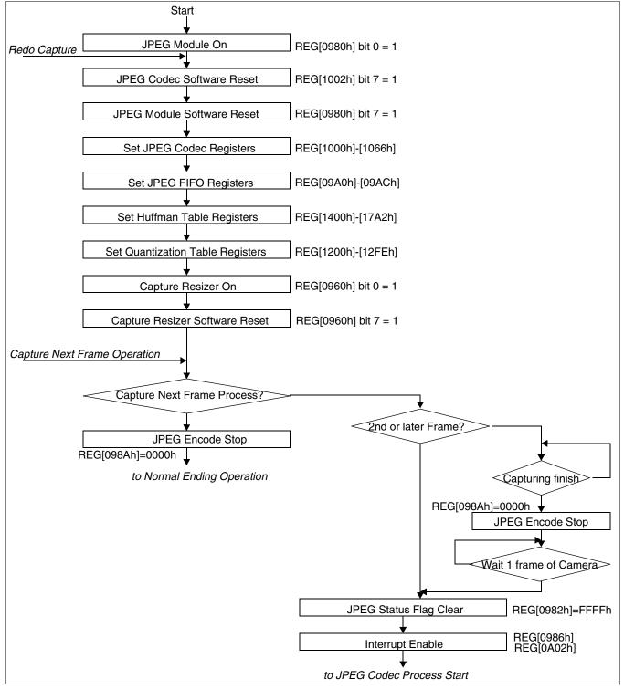
Figure 19-2: JPEG Encoding Process (1 of 4)
