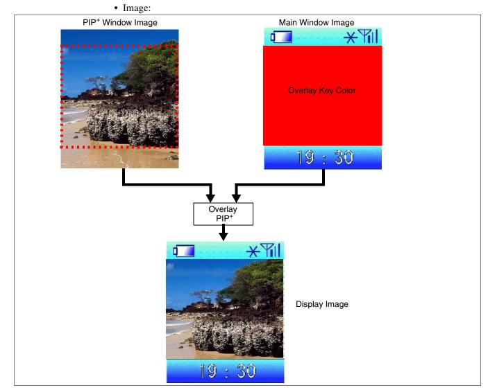
*Figure 8-5: Main Window, PIP*<sup>+</sup> *Window, and Overlay Display*
