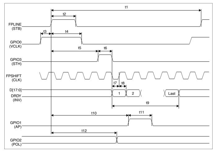
Figure 7-39: TFT Type 2 Horizontal Timing
