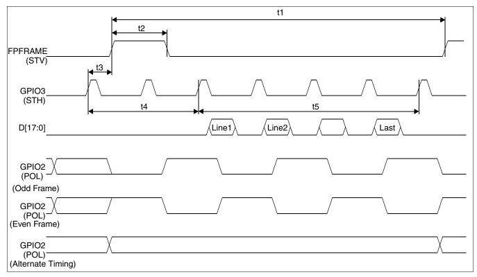
Figure 7-40: TFT Type 2 Vertical Timing
