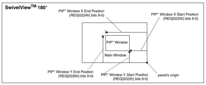
Figure 15-3: PIP<sup>+</sup> with SwivelView 180° Enabled
