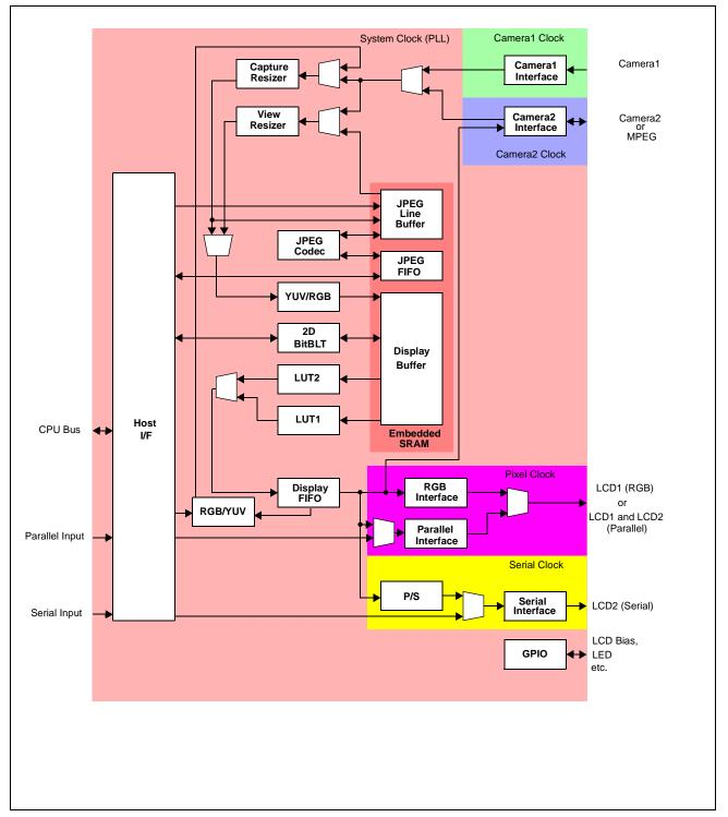
Figure 4-1: S1D13715 Block Diagram
