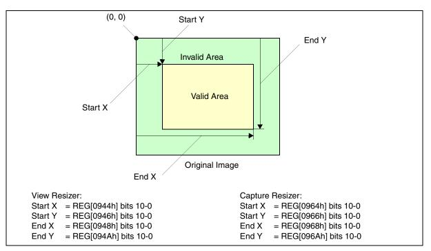
Figure 17-1: Trimming Function
