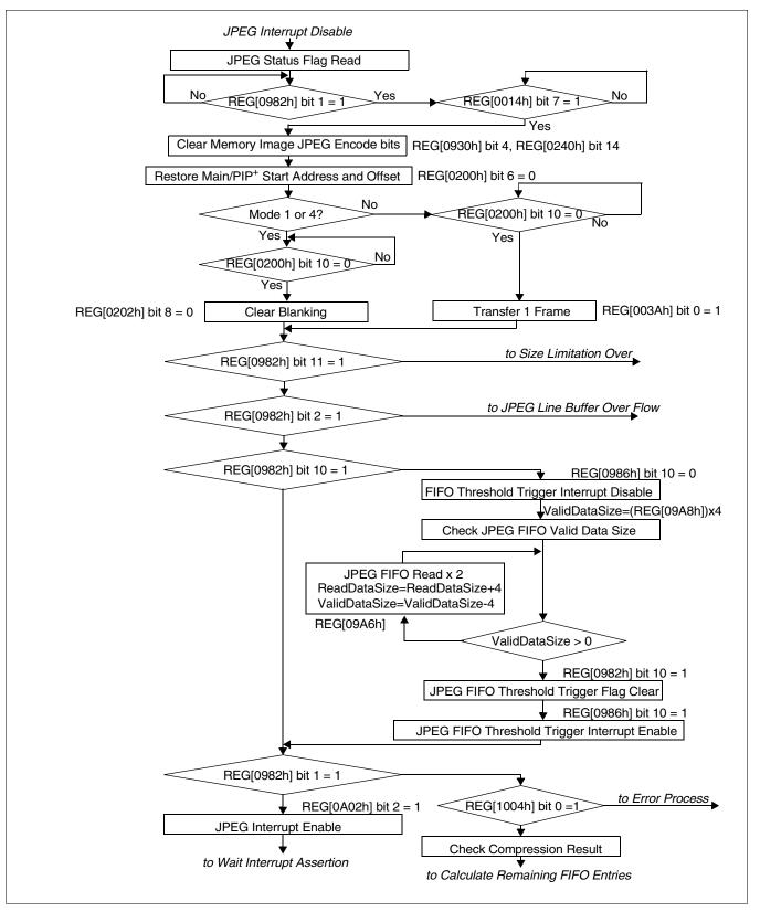
Figure 19-8: Memory Image JPEG Encoding Process (3 of 4)
