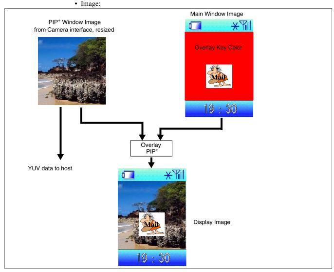
Figure 8-7: Main Window, PIP<sup>+</sup> Window, Overlay, and YUV
