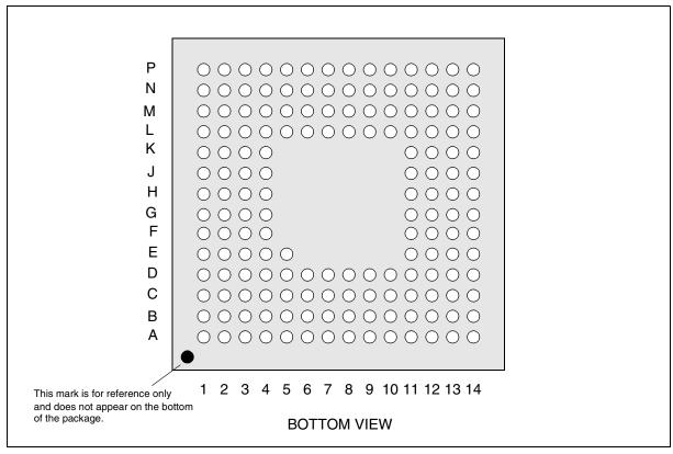
Figure 5-2: S1D13715 FCBGA-160 Pin Mapping
