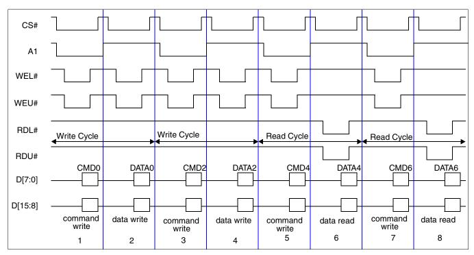
*Figure 21-1: Register Read/Write" Example Sequence*
