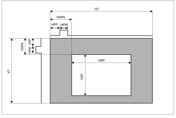
Figure 7-30: Generic TFT Panel Timing
