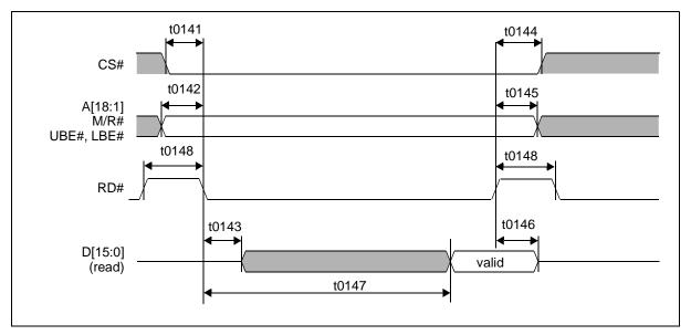
Figure 7-8: Direct 80 Type 1 Interface Read Cycle Timing (No Wait Mode)
