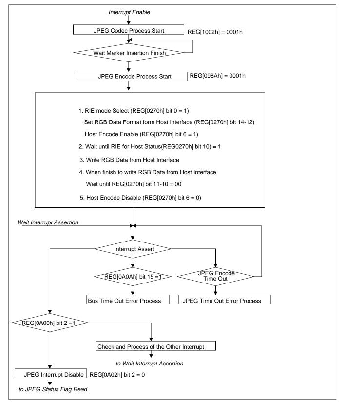
Figure 19-11: Memory Image JPEG Encoding Process from Host I/F (RGB format) (2 of 4)
