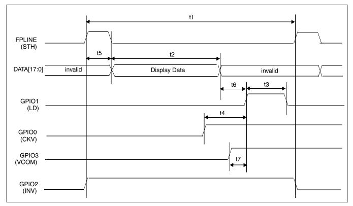
Figure 7-37: α-TFT Panel Horizontal Timing
