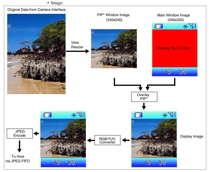
Figure 8-11: Main Window, PIP<sup>+</sup> Window, Overlay, RGB/YUV Converter and JPEG
