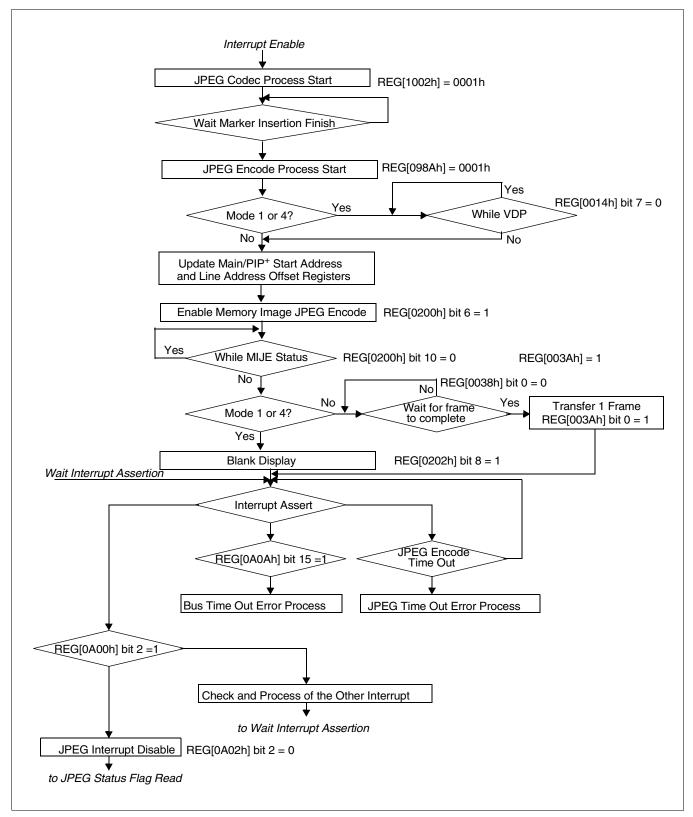
Figure 19-7: Memory Image JPEG Encoding Process (2 of 4)
