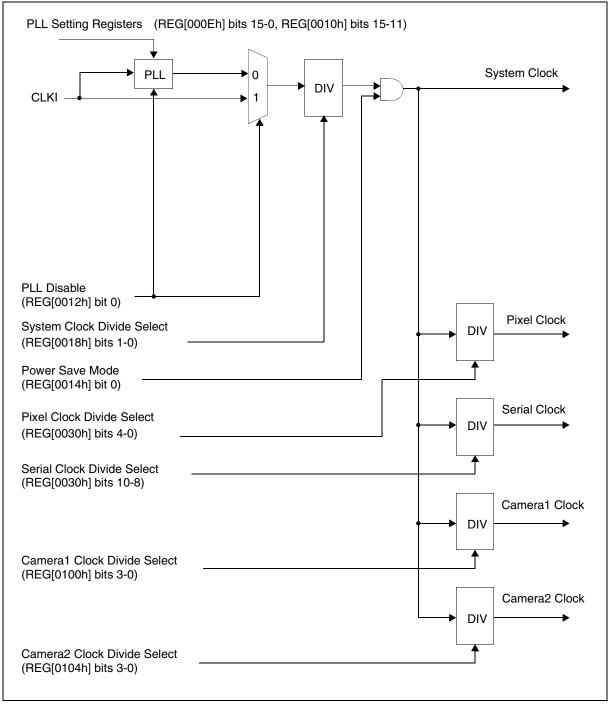
Figure 9-1: Clock Diagram
