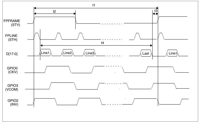
Figure 7-38: α–TFT Panel Vertical Timing
