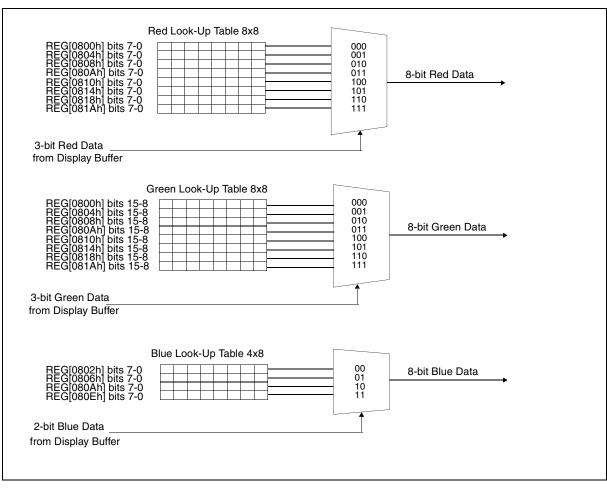
Figure 12-2: LUT2 (PIP<sup>+</sup> Window) for 8 Bpp Architecture
