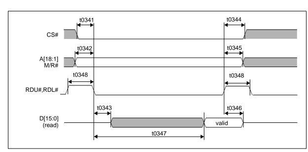
Figure 7-14: Direct 80 Type 3 Interface Read Cycle Timing (No Wait Mode)
