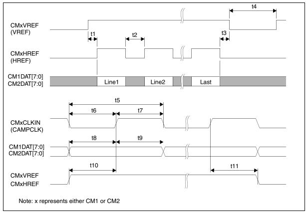
Figure 7-47: S1D13715B00 Camera Interface Timing
