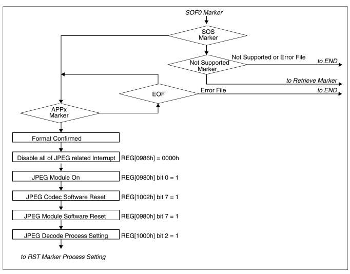
Figure 19-15: JPEG Decoding Process (2 of 6)
