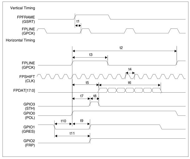
Figure 7-35: Casio TFT Horizontal Timing
