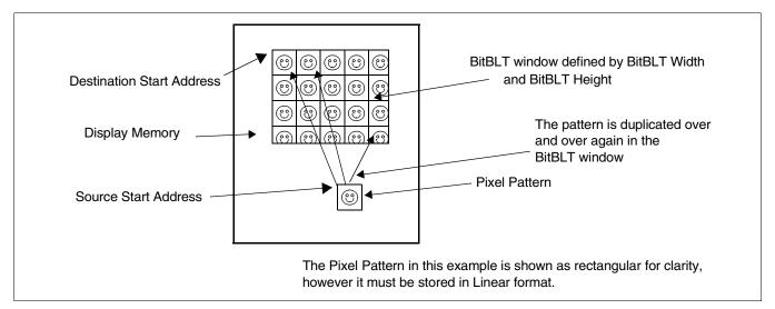
Figure 16-3: Pattern Fill Drawing
