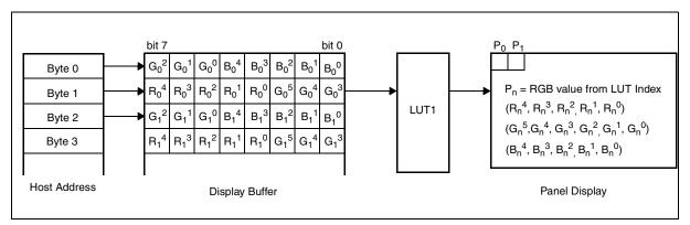
Figure 13-3: LUT1 for 16 Bpp Mode
