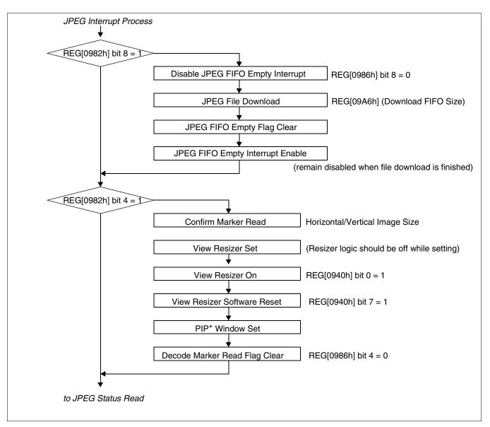
Figure 19-18: JPEG Decoding Process (5 of 6)
