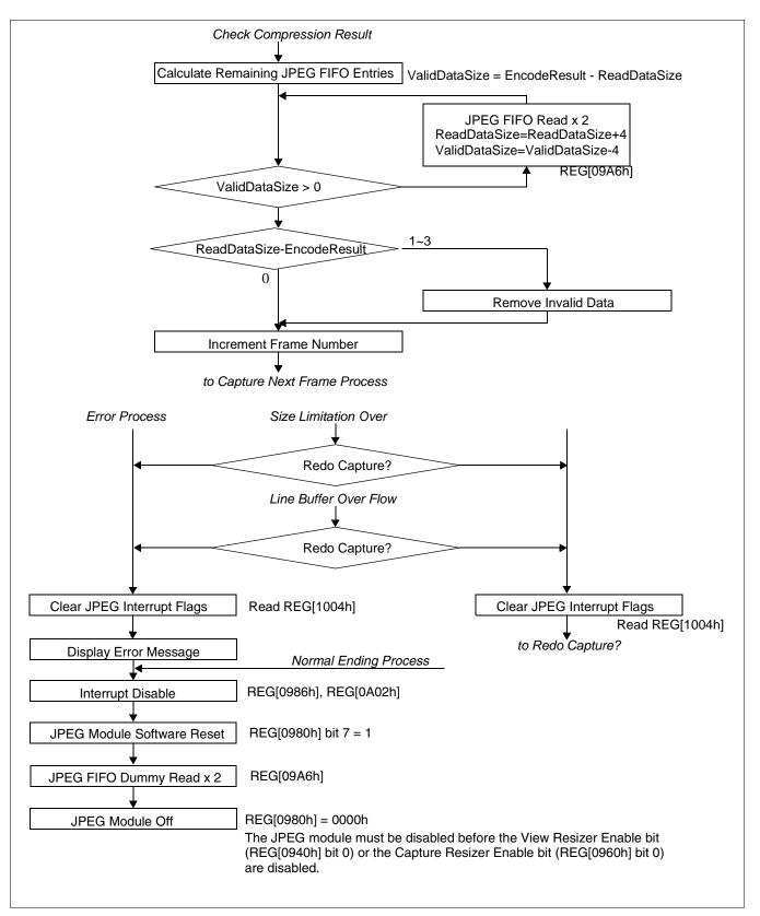
Figure 19-5: JPEG Encoding Process (4 of 4)
