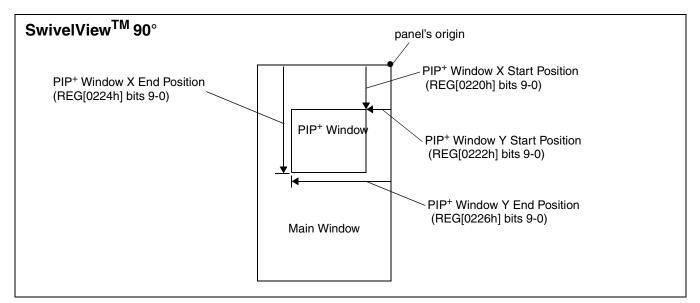
*Figure 15-2: PIP*<sup>+</sup> *with SwivelView 90*° *Enabled*
