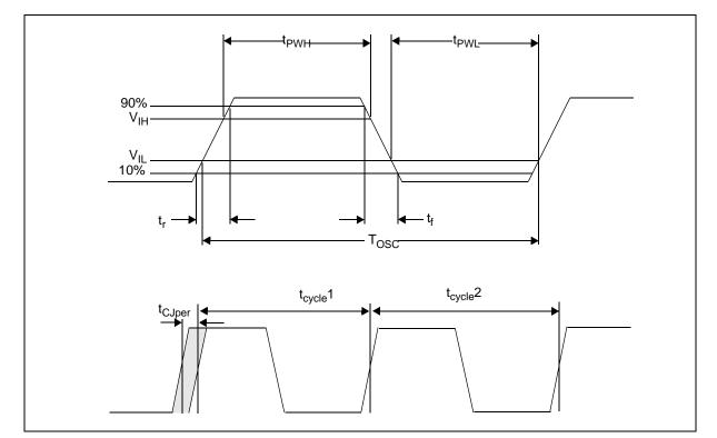
Figure 7-1: Clock Input Requirements (PLL)
