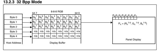
Figure 13-7: LUT Bypass for 32 bpp Mode
