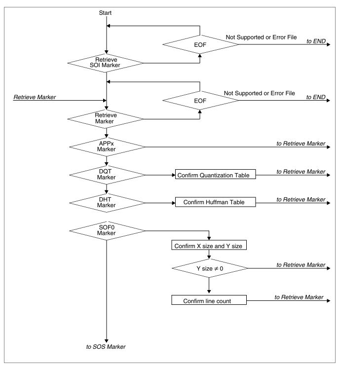
Figure 19-14: JPEG Decoding Process (1 of 6)
