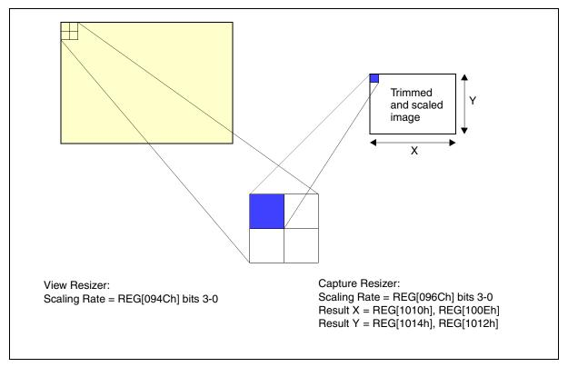
Figure 17-2: Scaling Example (1/2 Scaling)
