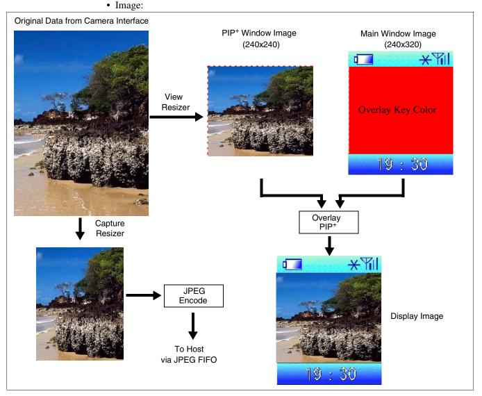
Figure 8-9: Main Window, PIP<sup>+</sup> Window, Overlay, and JPEG
