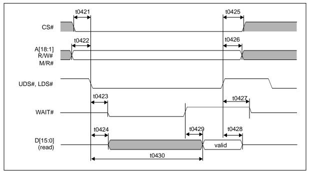
Figure 7-16: Direct 68 Interface Read Cycle Timing (Wait Mode)
