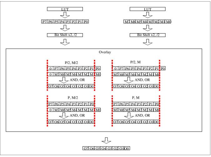
The following table shows the resulting PIP<sup>+</sup> window color when overlay is combined with the PIP<sup>+</sup> Window Bit Shift and the Main Window Bit Shift functions.
