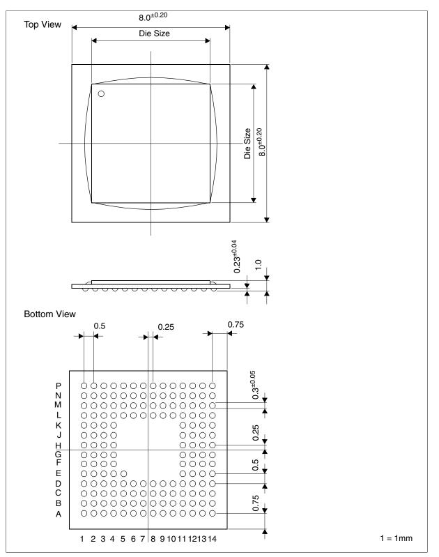
Figure 22-2: S1D13715 FCBGA 160-Pin Package
