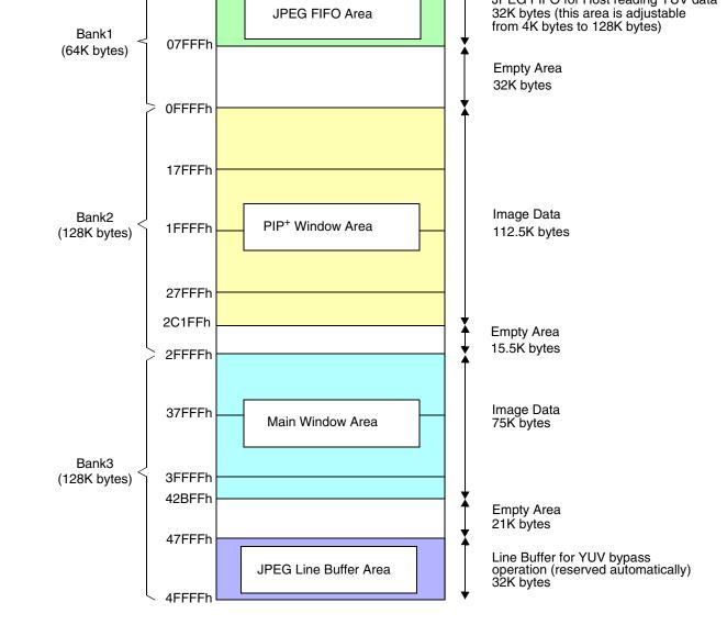
Figure 8-8: Memory Map for Main Window, PIP<sup>+</sup> Window, Overlay, and YUV
