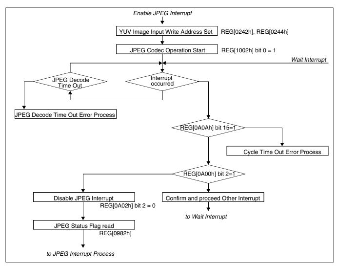
Figure 19-17: JPEG Decoding Process (4 of 6)
