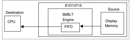
Figure 16-1: Read BitBLT Data Flow
