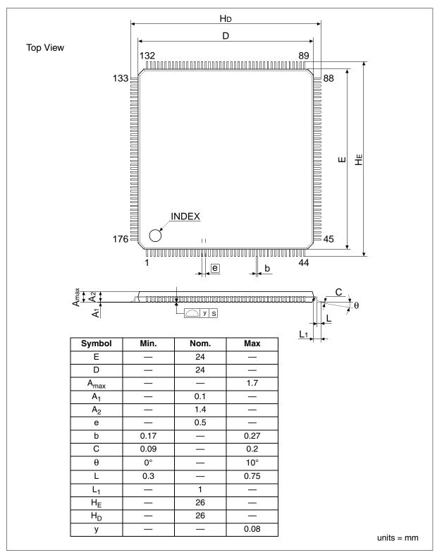
Figure 22-3: S1D13715 QFP21 176-Pin Package
