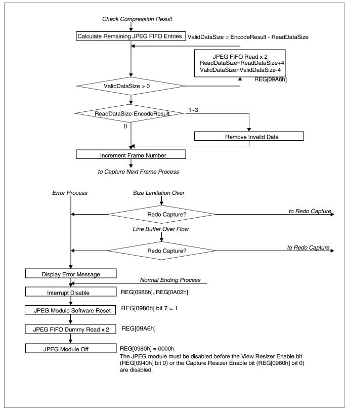
Figure 19-9: Memory Image JPEG Encoding Process (4 of 4)
