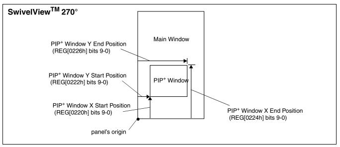
*Figure 15-4: PIP*<sup>+</sup> *with SwivelView 270° Enabled*
