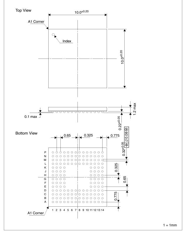
Figure 22-1: S1D13715 PFBGA 160-pin Package
