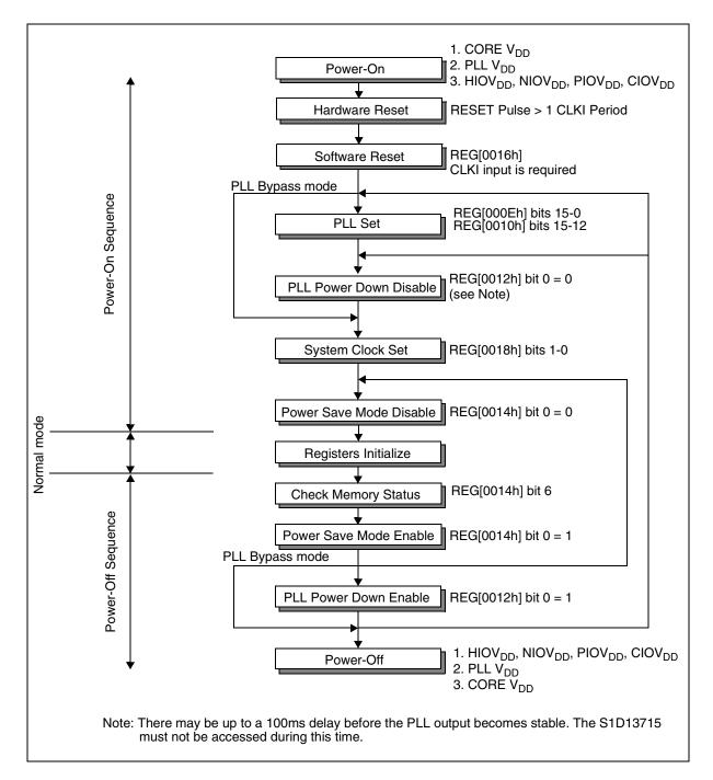
Figure 11-1: Power-On/Power-Off Sequence
