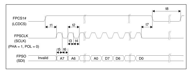
Figure 7-44: LCD1 uWIRE Serial Interface Timing
