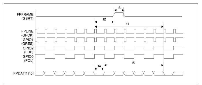
Figure 7-36: Casio TFT Vertical Timing
