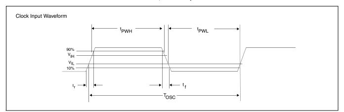
Figure 7-2: Clock Input Requirements (PLL bypassed)
