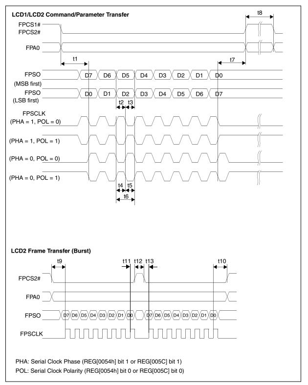
Figure 7-41: LCD1 ND-TFD, LCD2 8-Bit Serial Interface Timing
