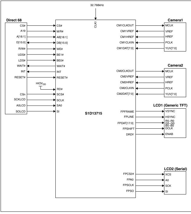
Figure 3-1: S1D13715 System Diagram 1
