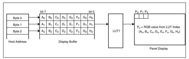
Figure 13-1: LUT1 for 8 Bpp Mode
