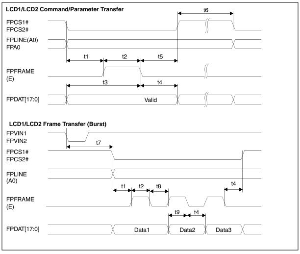
Figure 7-46: LCD1, LCD2 Parallel Interface Timing (68)
