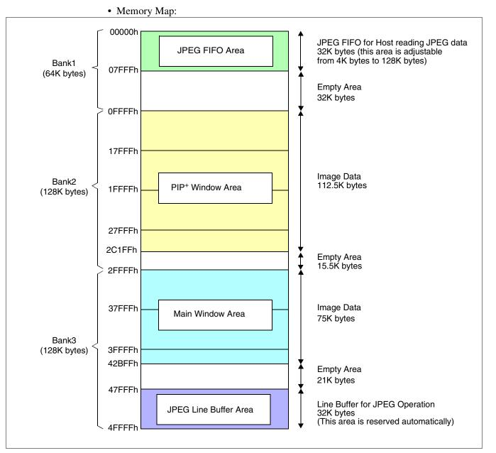
Figure 8-12: Memory Map for Main Window, PIP<sup>+</sup> Window, Overlay, RGB/YUV Converter and JPEG
