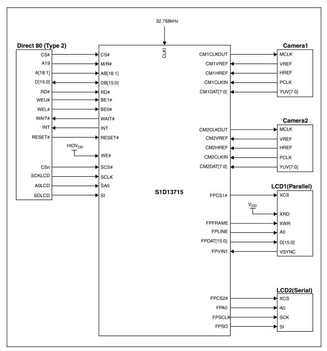
Figure 3-3: S1D13715 System Diagram 3
