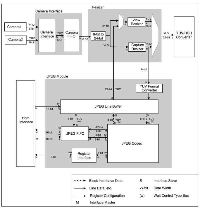
The following is an overview block diagram of how the digital video functions interact.
