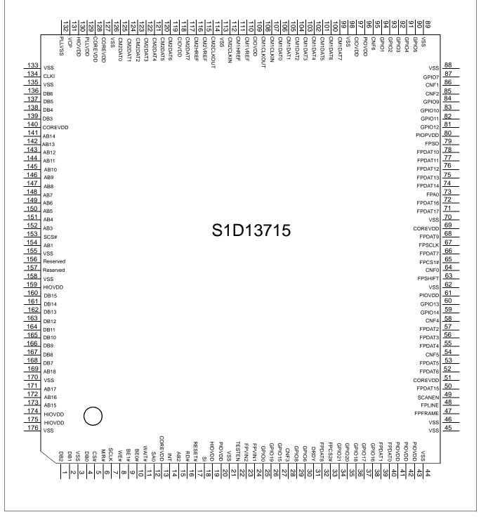
Figure 5-3: S1D13715 QFP21-176 Pin Mapping (Top View)
