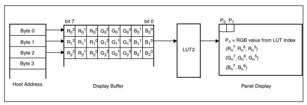
Figure 13-2: LUT2 for 8 Bpp Mode
