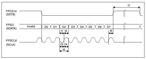
Figure 7-43: LCD1 a-Si TFT Serial Interface Timing
