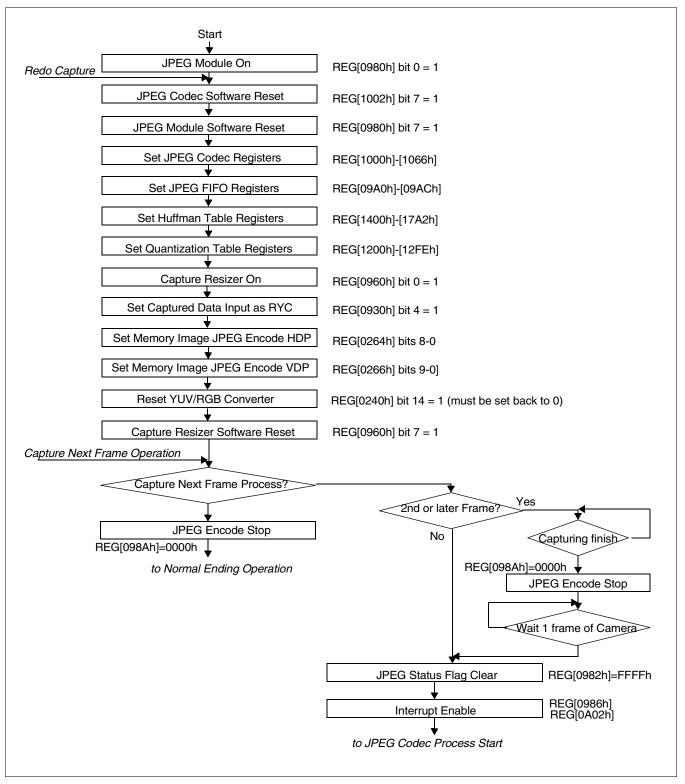
Figure 19-6: Memory Image JPEG Encoding Process (1 of 4)
