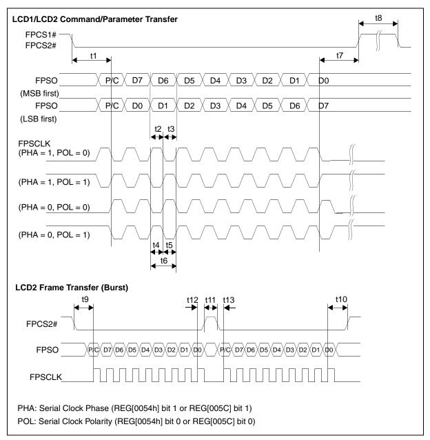
Figure 7-42: LCD1 ND-TFD, LCD2 9-Bit Serial Interface Timing
