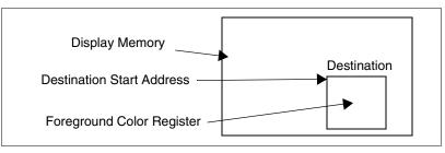
Figure 16-4: Solid Fill BitBLT Data Flow
