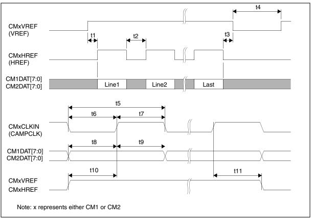
Figure 7-48: S1D13715B01 Camera Interface Timing
