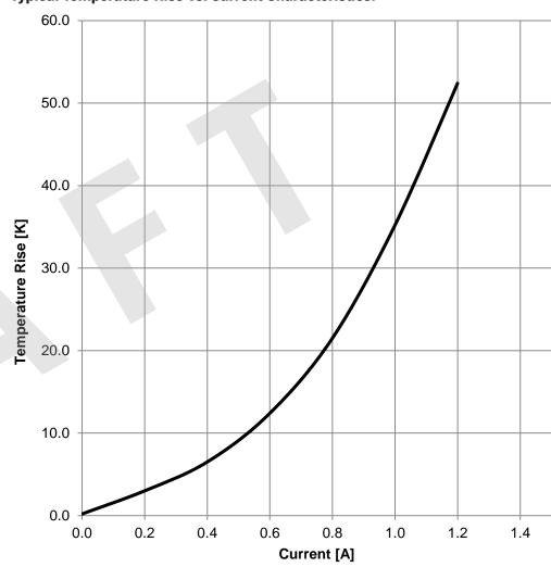
CHECKED GENERAL TOLERANCE CREATED Würth Elektronik eiSos GmbH & Co. KG EMC & Inductive Solutions KaS CSo DIN ISO 2768-1m Max-Eyth-Str. 1 74638 Waldenburg **WE-WPCC Wireless Power** Tel. +49 (0) 79 42 945 - 0 **Charging Receiver Coil** ORDER CODE www.we-online.com 760308101214 eiSos@we-online.com DATE (YYYY-MM-DD) BUSINESS UNIT REVISION PAGE 001.001 2017-04-24 3/6 Valid **WÜRTH ELEKTRONİK**
