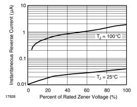
Fig. 5 - Typical Reverse Characteristics
