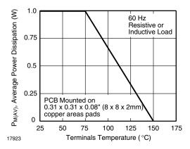
Fig. 1 - Maximum Continuous Power Dissipation
