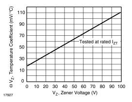
Fig. 3 - Typical Temperature Coefficients
