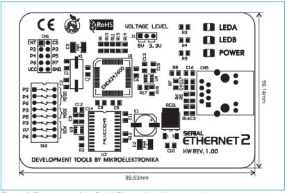
Figure 2: Dimensions of the Serial Ethernet2 additional board
