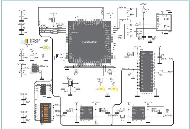
Figure 3: Serial Ethernet2 board connection schematic
