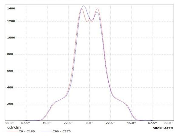
Luminaire: Ledil Oy CN12351\_Brooke-SCR-W\_L230 LOR=90% Lamps: 1 x Citizen CL-L233 280Im 250mA
