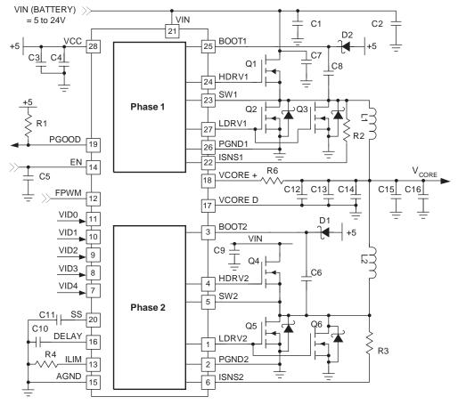
Figure 1. AMD Mobile Athlon/Duron CPU Core Supply
