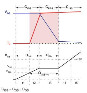
Figure 12. Switching losses and Q<sub>G</sub>
