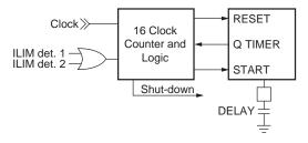
Figure 10. Over-Current Shut-Down Delay Logic
