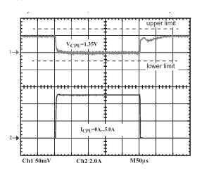
Figure 8. Converter Response to 5A Load Step
