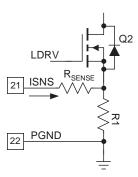
Figure 11. Improving current sensing accuracy
