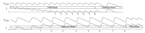
Figure 4. Transitioning between PWM and Hysteretic Mode
