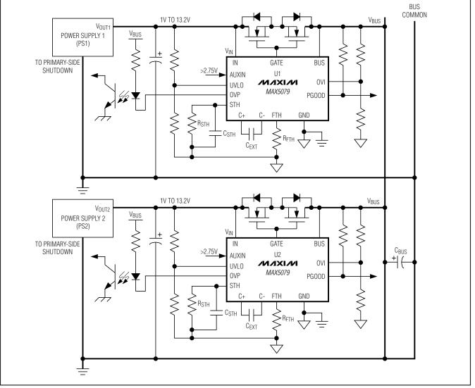
Figure 3. Parallel Supplies with Back-to-Back MOSFET
