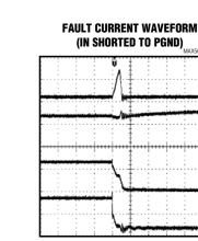
$\begin{array}{l} 1\mu s/div \\ V_{IN}=2.75V, \ V_{BUS}=2.75V, \\ V_{AUXIN}=0V, \ C_{STH}=0\mu F, \\ R_{STH}=0PEN, \ R_{FTH}=0, \\ UVLO=IN \end{array}$
