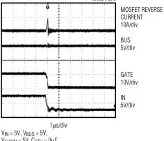
$\begin{array}{l} V_{IN}=5V, \ V_{BUS}=5V, \\ V_{AUXIN}=5V, \ C_{STH}=0\mu F, \\ R_{STH}=0PEN, \ R_{FTH}=0, \\ UVL0=IN \end{array}$
