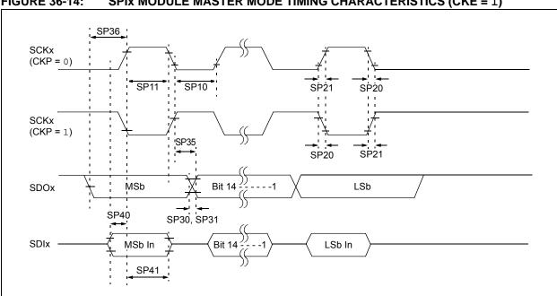
FIGURE 36-14: SPIX MODULE MASTER MODE TIMING CHARACTERISTICS (CKE = 1)
