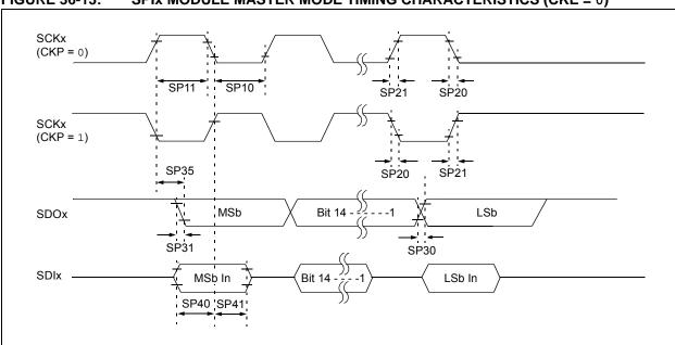
FIGURE 36-13: SPIX MODULE MASTER MODE TIMING CHARACTERISTICS (CKE = 0)
