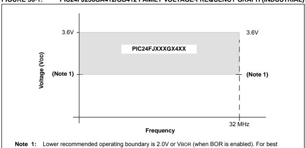
Note 1: Lower recommended operating boundary is 2.0V or VBOR (when BOR is enabled). For besi analog performance, operation above 2.2V is suggested, but not required.
