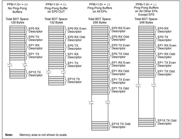
BDs have a fixed relationship to a particular endpoint, depending on the buffering configuration. Table 20-2 provides the mapping of BDs to endpoints. This relationship also means that gaps may occur in the BDT if endpoints are not enabled contiguously. This, theoretically, means that the BDs for disabled endpoints could be used as buffer space. In practice, users should avoid using such spaces in the BDT unless a method of validating BD addresses is implemented.
