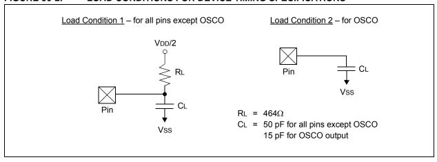
TABLE 36-19: CAPACITIVE LOADING REQUIREMENTS ON OUTPUT PINS
