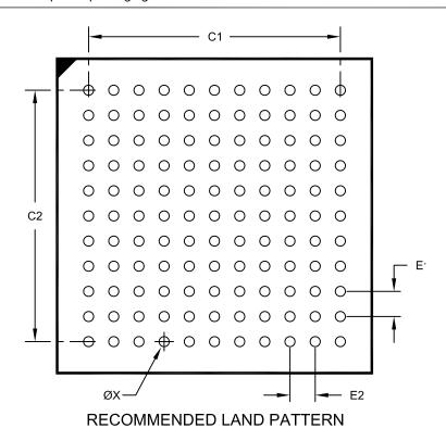
Units MILLIMETERS **Dimension Limits** MIN NOM MAX Contact Pitch 0.80 BSC E1 Contact Pitch E2 0.80 BSC Contact Pad Spacing C1 8.00 Contact Pad Spacing C2 8.00 Contact Pad Diameter (X121) Х 0.32
