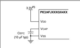
Note 1: This is a typical operating voltage. Refer to Section 36.0 "Electrical Characteristics" for the full operating ranges of VDD.
