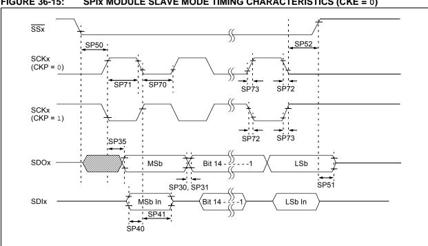
FIGURE 36-15: SPIX MODULE SLAVE MODE TIMING CHARACTERISTICS (CKE = 0)
