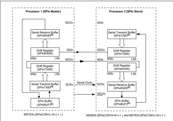
**Note 1:** Using the  $\overline{SSx}$  pin in Slave mode of operation is optional.
