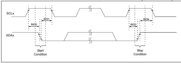
TABLE 36-30: I2Cx BUS START/STOP BITS TIMING REQUIREMENTS (MASTER MODE)
