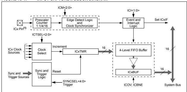
Note 1: The ICx inputs must be assigned to an available RPn/RPIn pin before use. See Section 11.5 "Peripheral Pin Select (PPS)" for more information.
