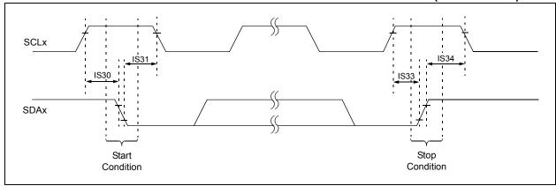
TABLE 36-32: I2Cx BUS START/STOP BITS TIMING REQUIREMENTS (SLAVE MODE)
