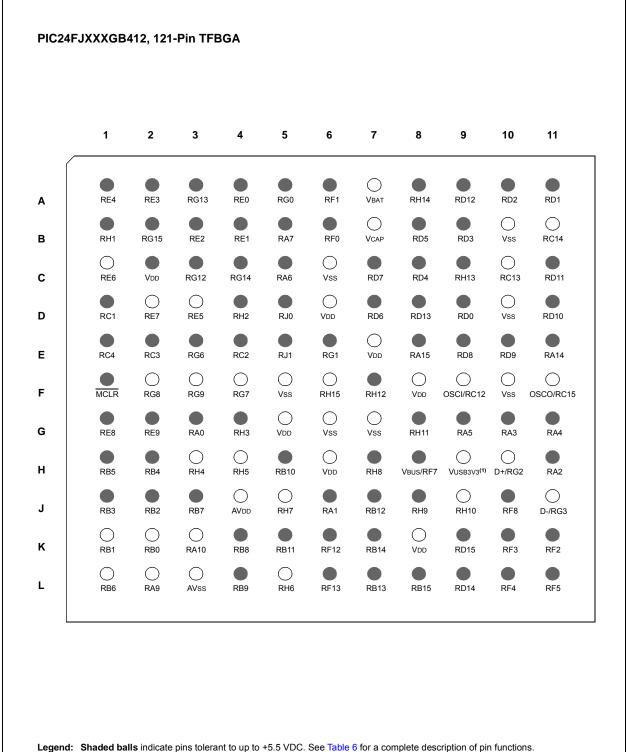
Legent. Shades bass indicate pins tolerant to up to +5.5 VDC. See Table 0 for a complete description of pin function
