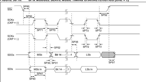
FIGURE 36-16: SPIX MODULE SLAVE MODE TIMING CHARACTERISTICS (CKE = 1)
