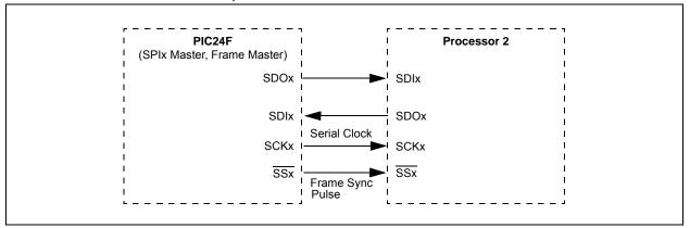
FIGURE 17-6: SPIX MASTER, FRAME SLAVE CONNECTION DIAGRAM
