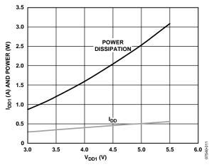
Figure 12. Typical Short-Circuit Input Current and Power vs. V<sub>DD1</sub> Supply Voltage
