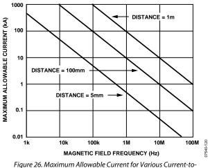
Figure 26. Maximum Allowable Current for Various Current-to-ADuM5200/ADuM5201/ADuM5202 Spacings
