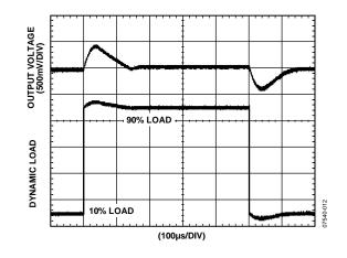
Figure 13. Typical V<sub>Iso</sub> Transient Load Response, 5 V Output, 10% to 90% Load Step
