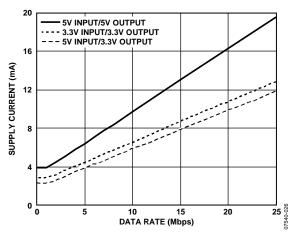
Figure 20. Typical I<sub>CHn</sub> Supply Current per Reverse Data Channel (15 pF Output Load)
