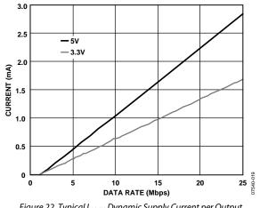
Figure 22. Typical I<sub>ISO(D)</sub> Dynamic Supply Current per Output (15 pF Output Load)
