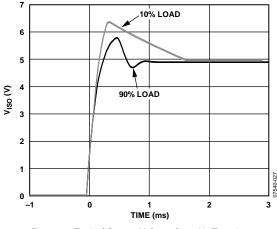
Figure 17. Typical Output Voltage Start-Up Transient at 10% and 90% Load,  $V_{\rm ISO}$  = 5 V
