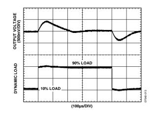
Figure 14. Typical V<sub>ISO</sub> Transient Load Response, 3 V Output, 10% to 90% Load Step
