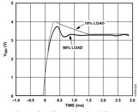
Figure 18. Typical Output Voltage Start-Up Transient at 10% and 90% Load, V<sub>ISO</sub> = 3.3 V
