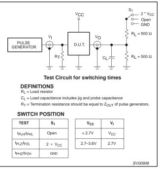
Waveform 5. Load circuitry for switching times
