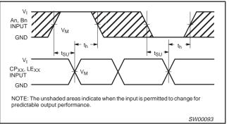
Waveform 4. Data set-up and hold times for the An and Bn inputs to the LE<sub>AB</sub>, LE<sub>BA</sub>,  $\overline{CP}_{AB}$  and  $\overline{CP}_{BA}$  inputs
