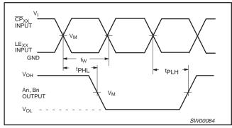
Waveform 2. Latch enable input (LE<sub>AB</sub>, LE<sub>BA</sub>) and clock pulse input ( $\overline{CP}_{AB}$ ,  $\overline{CP}_{BA}$ ) to output (An, Bn) propagation delays and latch enable pulse width
