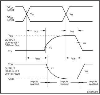
Waveform 3. 3-State enable and disable times
