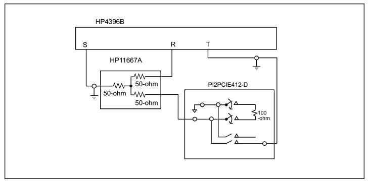
Fig 2. Off-isolation setup
