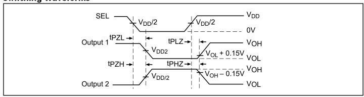
**Voltage Waveforms Enable and Disable Times**
