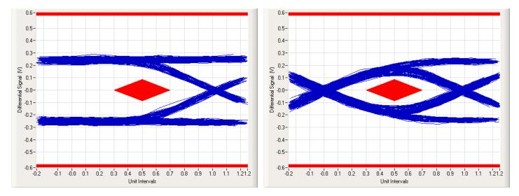
Figure 6: The worst non-transition signal eye (left) and the worst transition signal eye (right) of the PCI-SIG compliance software test using PI2PCIE412-D + 22.5" test card
