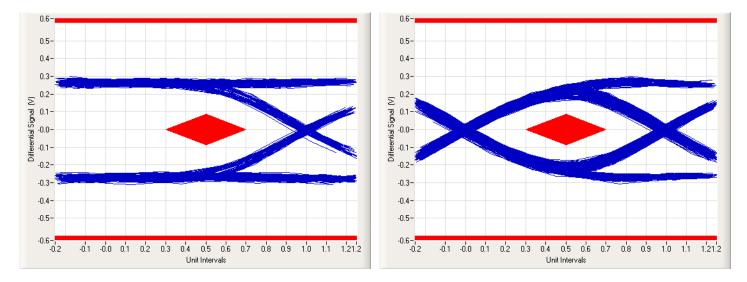
Figure 7. The worst non-transition signal eye (left) and the worst transition signal eye (right) of the PCI-SIG compliance software test with no switch + w/22.5" test card
