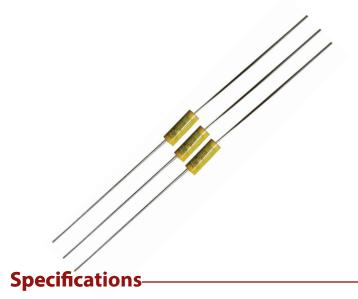
Type WMC axial-leaded polyester film/foil capacitors are ideal for automatic insertion in printed circuit boards. It is an ultraminiature version of Type WMF and the sections of these non-inductive capacitors are constructed with extended foil, polyester film, with tinned copper-clad steel leads.
