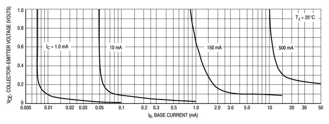
Figure 4. Collector Saturation Region
