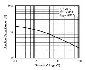
Fig. 5 - Typical Junction Capacitance
