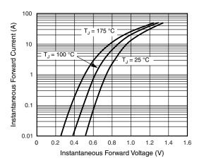
Fig. 3 - Typical Forward Voltage
