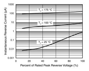
Fig. 4 - Typical Reverse Leakage Characteristics
