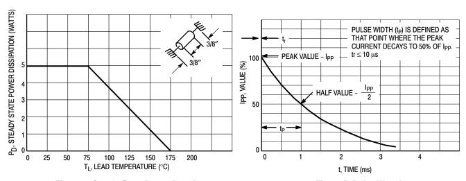
Figure 4. Steady State Power Derating
