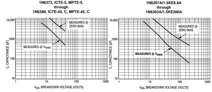
Figure 3. Capacitance versus Breakdown Voltage
