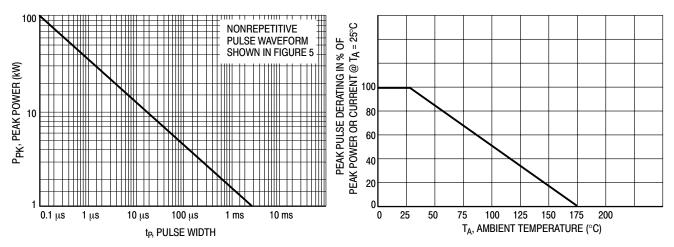
Figure 1. Pulse Rating Curve
