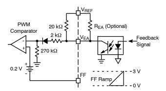
Figure 45. Optocoupler Driving V<sub>EA</sub> Input
