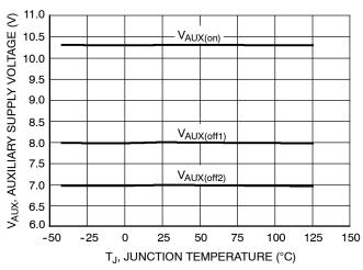
Figure 3. Auxiliary Supply Voltage Thresholds vs. Junction Temperature
