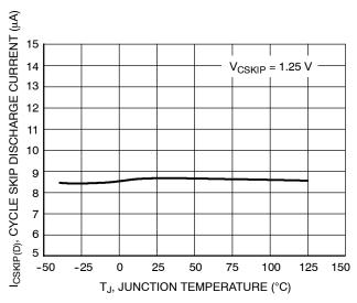
Figure 19. Cycle Skip Discharge Current vs. Junction Temperature
