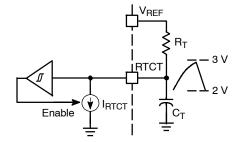
Figure 48. Oscillator Configuration
