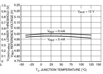
Figure 21. Reference Voltage vs. Junction Temperature
