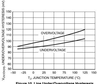
Figure 10. Line Under/Overvoltage Hysteresis vs. Junction Temperature
