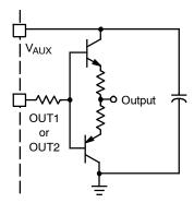
Figure 46. Discrete Boost Drive Stage
