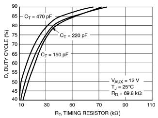
Figure 25. Duty Cycle vs. Timing Resistor
