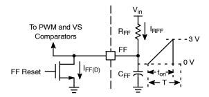
Figure 44. Feed Forward Ramp Generation
