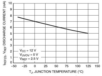
Figure 22. V<sub>REF</sub> Discharge Current vs. Junction Temperature
