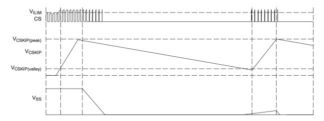
Figure 37. Cycle Skip Waveforms
