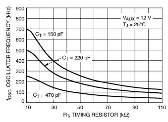
Figure 24. Oscillator Frequency vs. Timing Resistor
