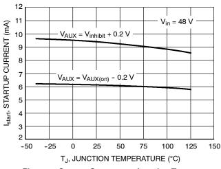
Figure 4. Startup Current vs. Junction Temperature
