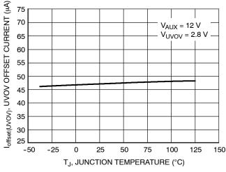
Figure 11. UVOV Offset Current vs. Junction Temperature
