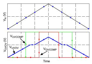
Figure 43. UVOV Detectors Typical Waveforms
