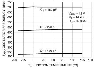
Figure 23. Oscillator Frequency vs. Junction Temperature
