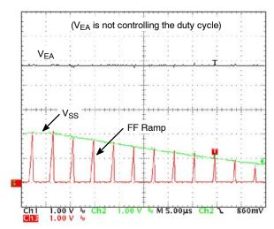
Figure 34. Soft-Stop Before Soft-Start is Complete and V<sub>EA</sub> is Open.
