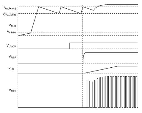
Figure 40. Startup Circuit Waveforms
