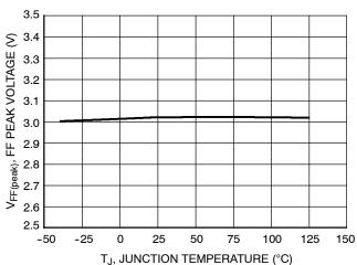
Figure 14. Feedforward Peak Voltage vs. Junction Temperature
