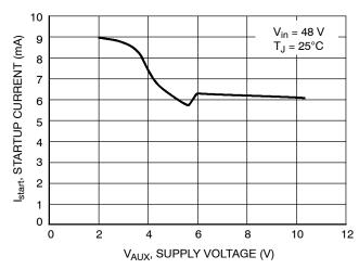
Figure 5. Startup Current vs. Supply Voltage
