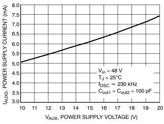
Figure 8. Supply Current vs. Supply Voltage
