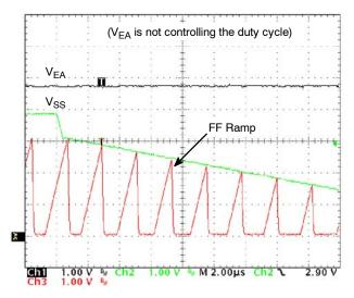
Figure 36. Soft-Stop Behavior After Soft-Start is Complete and V<sub>EA</sub> is Open.
