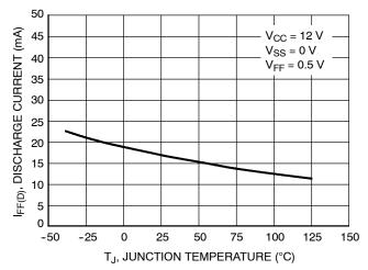
Figure 12. FF Discharge Current vs. Junction Temperature
