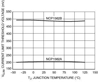
Figure 15. Current Limit Threshold Voltage vs. Junction Temperature
