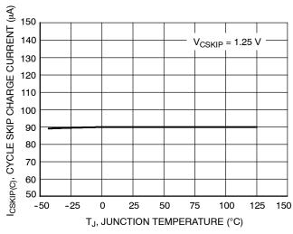
Figure 18. Cycle Skip Charge Current vs. Junction Temperature
