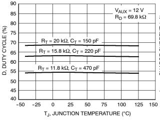
Figure 26. Duty Cycle vs. Junction Temperature
