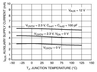
Figure 7. Auxiliary Supply Current vs. Junction Temperature
