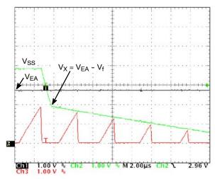
Figure 35. Soft-Stop Behavior when V<sub>EA</sub> Controls the Duty Cycle.
