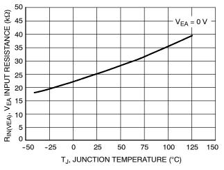
Figure 32. V<sub>EA</sub> Input Resistance vs. Junction Temperature
