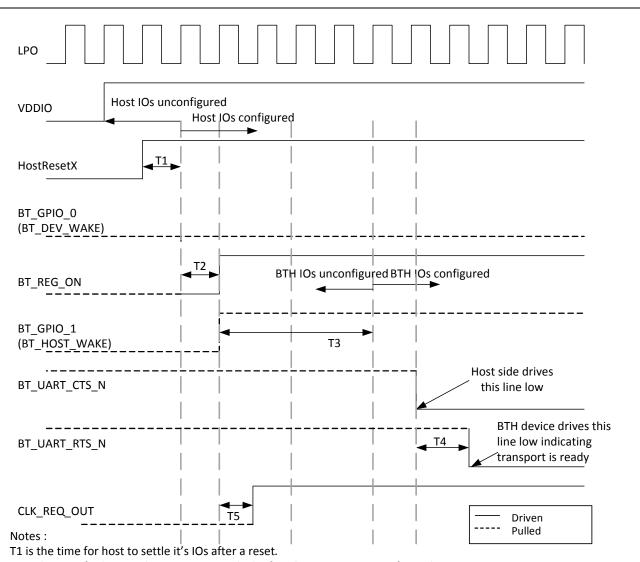
Figure 19. Startup Signaling Sequence
