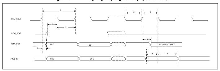
Table 12. PCM Interface Timing Specifications (Long Frame Sync, Slave Mode)
