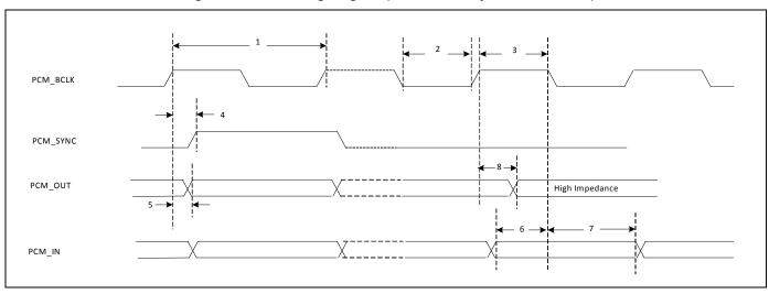
Table 9. PCM Interface Timing Specifications (Short Frame Sync, Master Mode)
