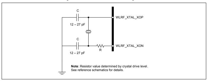
The CYW43438 uses a fractional-N synthesizer to generate the radio frequencies, clocks, and data/packet timing so that it can operate using numerous frequency references. The frequency reference can be an external source such as a TCXO or a crystal interfaced directly to the CYW43438.
