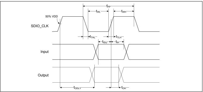
Table 43. SDIO Bus Timing <sup>1</sup> Parameters (High-Speed Mode)
