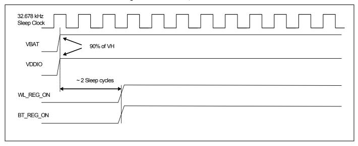
Figure 39. WLAN = OFF, Bluetooth = OFF
