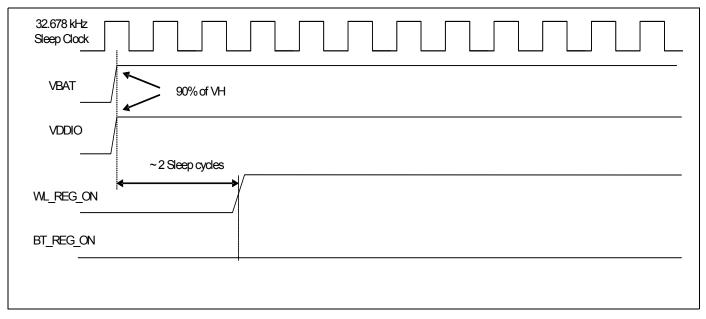
Figure 41. WLAN = OFF, Bluetooth = ON
