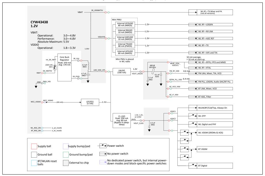
Figure 4. Typical Power Topology (2 of 2)
