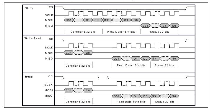
Figure 14. gSPI Signal Timing with Status (Response Delay = 0)
