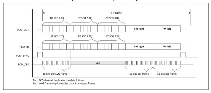
Figure 22. Functional Multiplex Data Diagram
