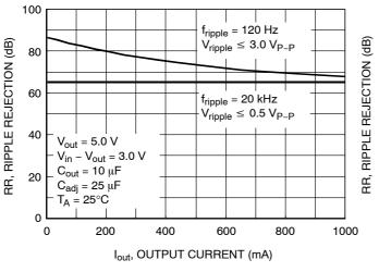
Figure 10. NCP1117XTA Ripple Rejection vs. Output Current
