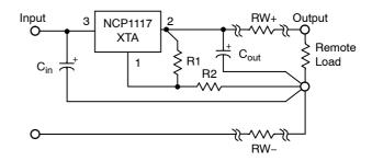
Figure 26. Load Sensing
