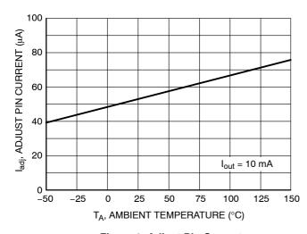
Figure 8. Adjust Pin Current vs. Temperature
