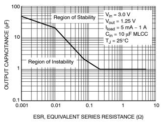
Figure 12. Output Capacitance vs. ESR
