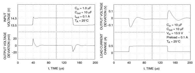
Figure 19. NCP1117XT12 Line Transient Response
