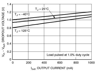
Figure 5. Dropout Voltage vs. Output Current
