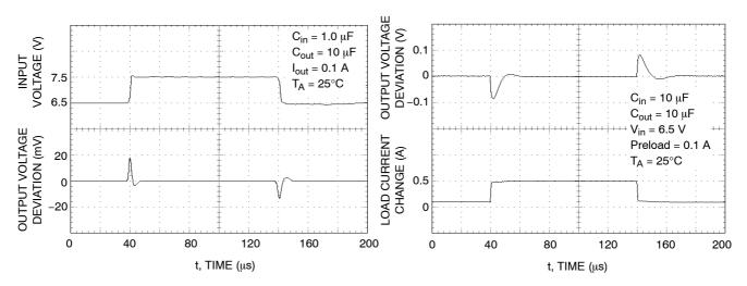
Figure 17. NCP1117XT50 Line Transient Response
