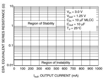
Figure 13. Typical ESR vs. Output Current
