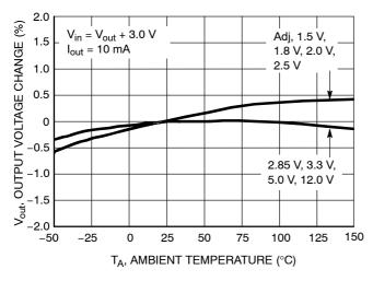
Figure 4. Output Voltage Change vs. Temperature
