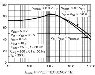
Figure 11. NCP1117XTA Ripple Rejection vs. Frequency
