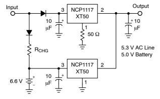
The 50  $\Omega$  resistor that is in series with the ground pin of the upper regulator level shifts its output 300 mV higher than the lower regulator. This keeps the lower regulator off until the input source is removed.
