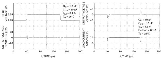
Figure 15. NCP1117XT285 Line Transient Response
