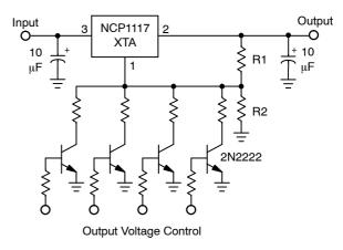
Resistor R2 sets the maximum output voltage. Each transistor reduces the output voltage when turned on.
