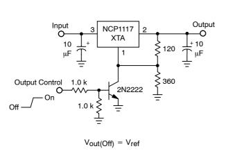
Figure 29. Regulator with Shutdown
