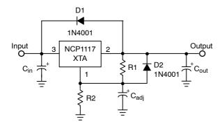
Figure 25. Protection Diode Placement
