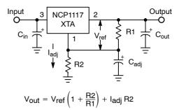
Figure 24. Adjustable Output Regulator
