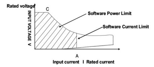
Note the gap between the operating region and the current axis for lower voltages. More detail is described in the following section.
