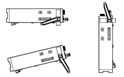
The handle may be removed if desired. A rack mounting kit (IT-E151) is also available for models 8500, 8502, 8510, 8512, 8514, and 8518.
