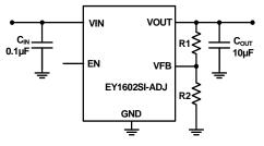
FIGURE 11. SETTING OUTPUT VOLTAGE
