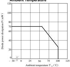
Fig. 3 Power Dissipation vs. Ambient Temperature
