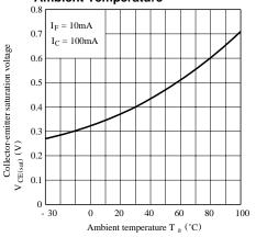
Fig.9 Collector-emitter Saturation Voltage vs. Ambient Temperature
