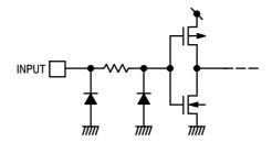
Figure 8. Input Equivalent Circuit
