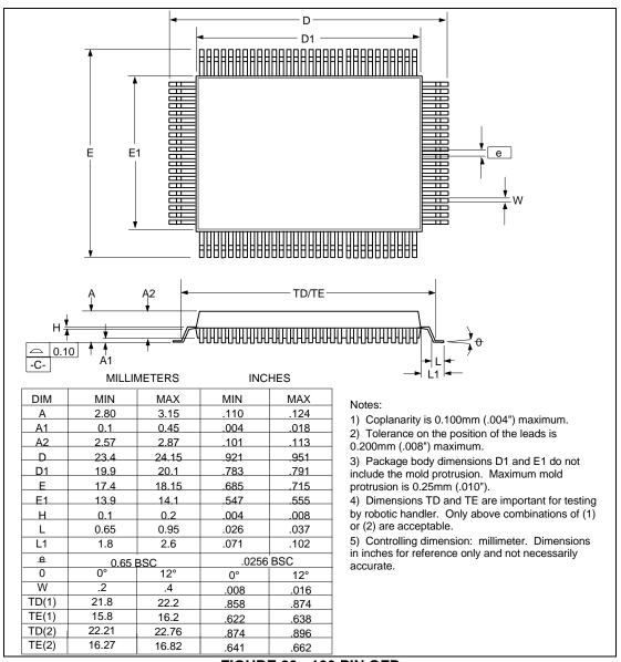
FIGURE 20 - 100 PIN QFP
