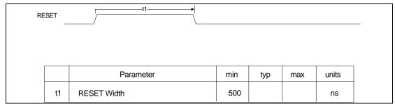
FIGURE 7 - RESET TIMING
