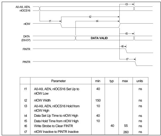
FIGURE 5 - MICROPROCESSOR WRITE TIMING
