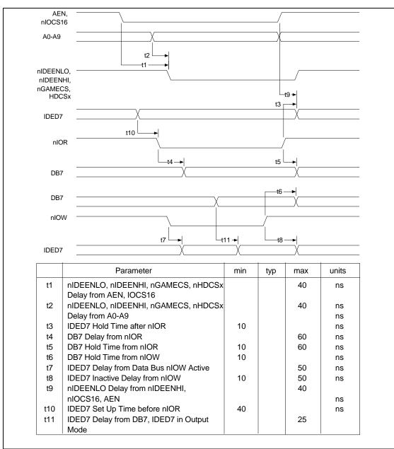
FIGURE 11 - IDE INTERFACE TIMING
