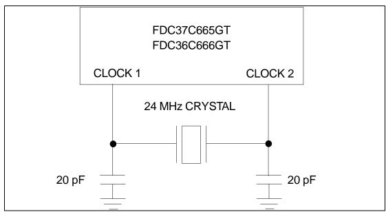
FIGURE 2 - SUGGESTED 24 MHz OSCILLATOR CIRCUIT
