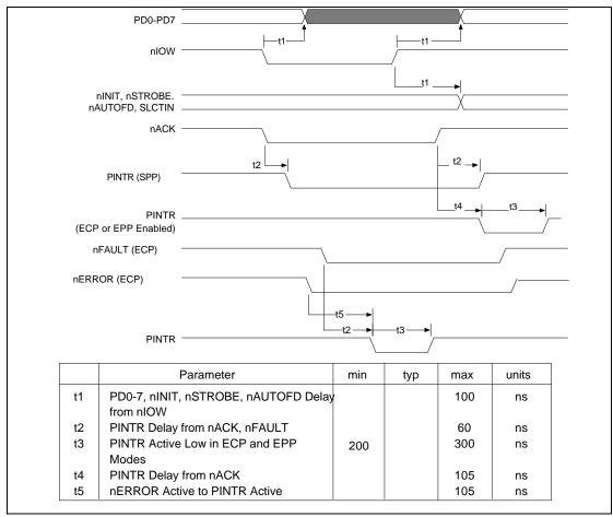
FIGURE 12 - PARALLEL PORT TIMING
