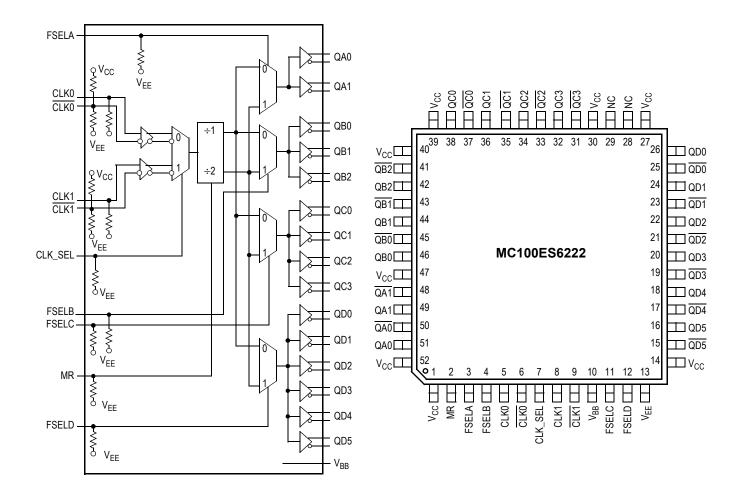
Figure 1. MC100ES6222 Logic Diagram
