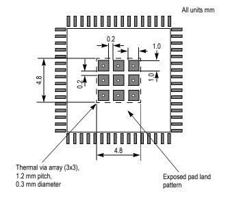
Figure 8. Recommended Solder Mask Openings
