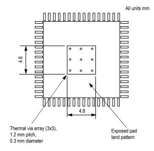
Figure 7. Recommended Thermal Land Pattern
