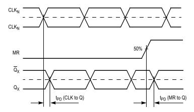
Figure 4. MC100ES6222  $t_{\mbox{\scriptsize PD}}$  Measurement Waveform
