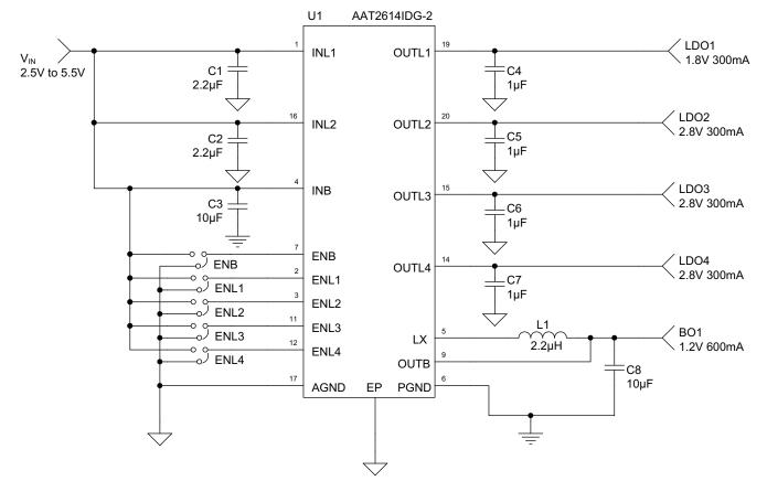
Figure 1: AAT2614IDG-2 Evaluation Board Schematic.
