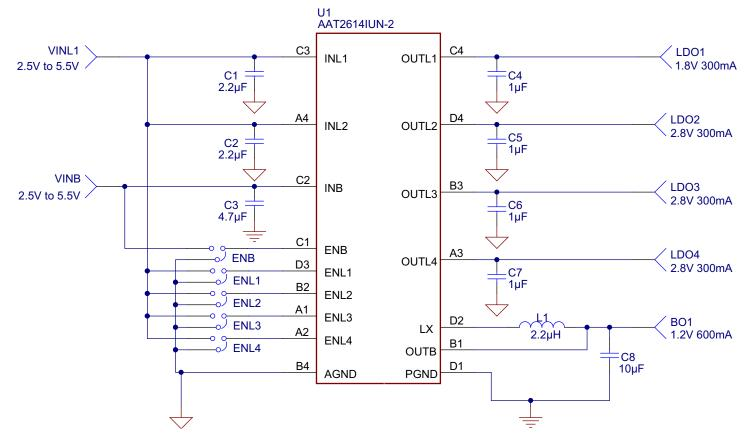
Figure 3: AAT2614IUN-2 Evaluation Board Schematic.
