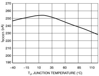
Figure 26. Pin 3 Source Current when (V<sub>OUT</sub> Low **Detect Threshold) is Activated vs. Temperature**
