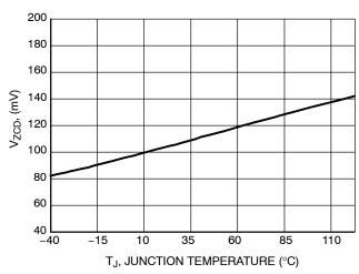
Figure 45. Pin 6 Comparator Threshold vs. Temperature
