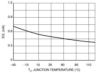
Figure 17. High-Voltage Current Source vs. Temperature (@ $V_{CC} = 0 V$ )
