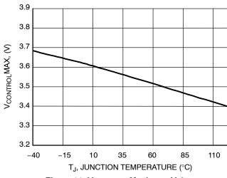
Figure 23. V<sub>CONTROL</sub> Maximum Voltage vs. Temperature
