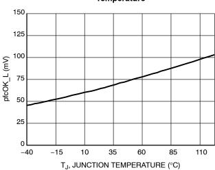
Figure 30. pfcOK Pin Low Level Voltage vs. **Temperature**
