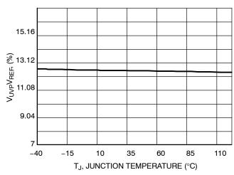
Figure 8. Ratio (V<sub>UVP</sub>/V<sub>REF</sub>) vs. Temperature
