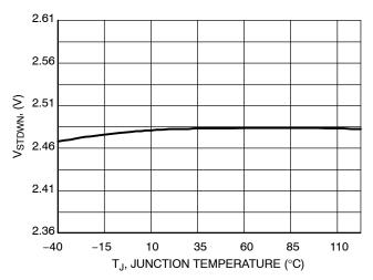
Figure 6. Shutdown Threshold vs. Temperature
