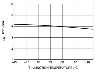
Figure 33. Operating Consumption vs. Temperature (V<sub>CC</sub> = 16 V, No Load, Switching)
