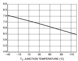
Figure 12. V<sub>CC</sub> Threshold Below which the Startup Current Source Turns on vs. Temperature
