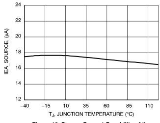
Figure 19. Source Current Capability of the Error Amplifier vs. Temperature
