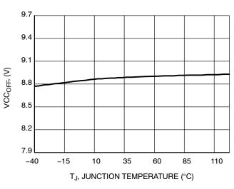
Figure 10. V<sub>CC</sub> Minimum Operating Voltage After Turn On – NCP1605/B
