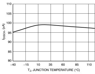
Figure 28. Oscillator Discharge Current vs. **Temperature**
