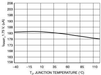
Figure 41. Pin 7 Source Current @ V<sub>PIN4</sub> = 1.75 V vs. Temperature
