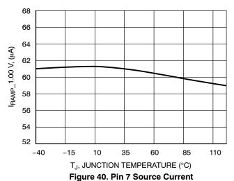
@ V<sub>PIN4</sub> = 1.0 V vs. Temperature
