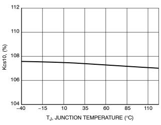
Figure 44. Ratio ( $I_{PIN6}$  /  $I_{PIN5}$ ) @  $I_{PIN5}$  = 10  $\mu A$  vs. Temperature
