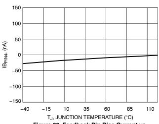
Figure 22. Feedback Pin Bias Current vs. Temperature (@ V<sub>PIN4</sub> = V<sub>REF</sub>)
