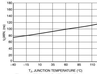
Figure 48. Minimum On-Time vs. Temperature
