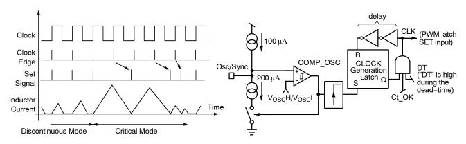
Figure 65. Oscillator Timing Diagram
