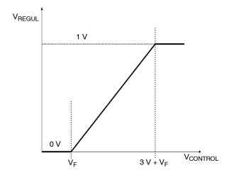
Figure 59. Correspondence between V<sub>CONTROL</sub> and V<sub>REGUL</sub>
