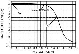
Figure 74. Startup Current vs.  $V_{CC}$  Voltage
