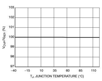
Figure 4. Overvoltage Threshold vs. Temperature
