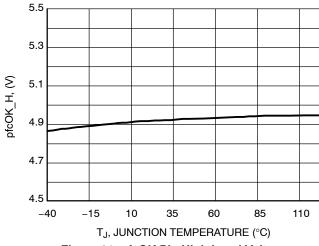
Figure 31. pfcOK Pin High Level Voltage vs. Temperature (250 μA Load)
