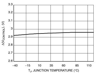
Figure 24.  $V_{CONTROL}$  Maximum Swing  $(\Delta V_{CONTROL})$  vs. Temperature
