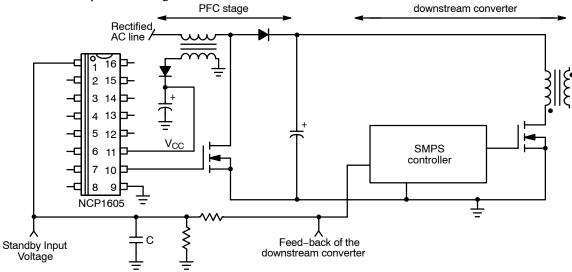
Figure 63. Signal for Standby Detection
