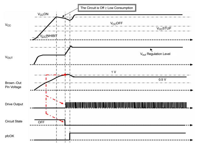
Figure 71. Startup and Brown Out Conditions
