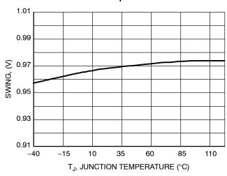
Figure 29. Oscillator Swing vs. Temperature
