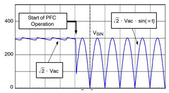
Figure 69. Typical Input Voltage of a PFC Stage
