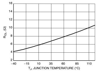
Figure 50. Gate Drive Sink Resistance vs. Temperature
