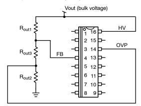
Figure 61. Configuration with One Feedback Network for Both OVP and Regulation
