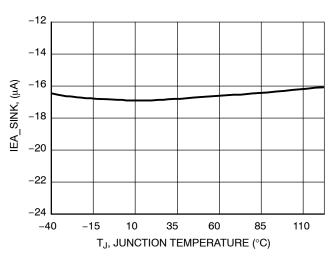
Figure 20. Sink Current Capability of the Error Amplifier vs. Temperature
