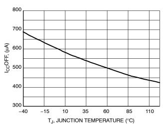
Figure 34. Off Mode Consumption vs. Temperature ( $V_{CC}$  = 16 V, Pin 2 Grounded)
