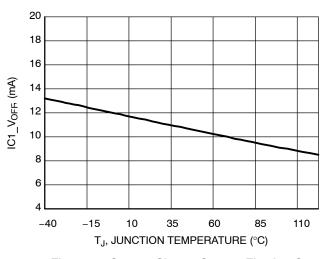
Figure 16. Startup Charge Current Flowing Out of the  $V_{CC}$  Pin vs. Temperature (@  $V_{CC}$  = 13.5 V)
