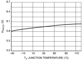
Figure 11. Difference (VCC<sub>ON</sub> – VCC<sub>OFF</sub>) vs. Temperature – NCP1605/B
