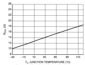
Figure 49. Gate Drive Source Resistance vs. Temperature
