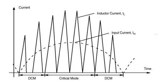
Figure 52. DCM and CRM Operation Within a Sinusoid Cycle
