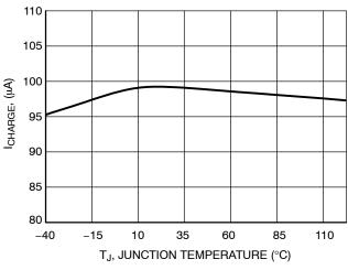
Figure 27. Oscillator Charge Current vs. **Temperature**
