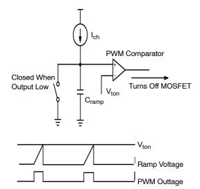
Figure 55. PWM Circuit and Timing Diagram
