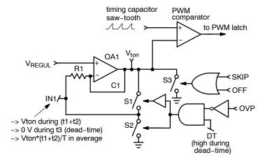
Figure 56. V<sub>TON</sub> Processing Circuit
