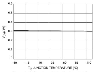
Figure 7. Undervoltage Protection Threshold vs. Temperature
