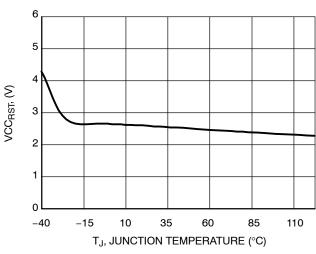
Figure 14. V<sub>CC</sub> Level Below Which the Logic Resets vs. Temperature
