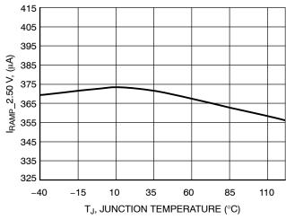
Figure 42. Pin 7 Source Current @ V<sub>PIN4</sub> = 2.5 V vs. Temperature
