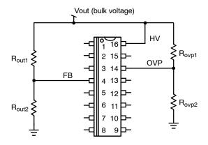
Figure 62. Configuration with Two Separate Feedback Networks
