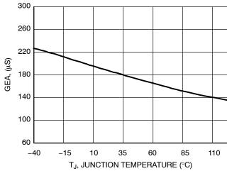
Figure 21. Error Amplifier Gain vs. Temperature
