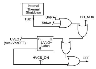
Figure 72. Fault Management Block
