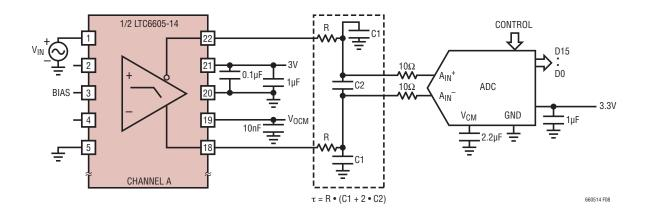
Figure 8. Driving an ADC
