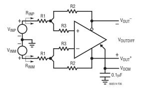
Figure 6. Input Impedance
