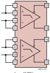
$f_{-3dB} = 12.3 MHz$ GAIN = 3V/V (9.5dB)  $Z_{IN} = 133 \Omega$
