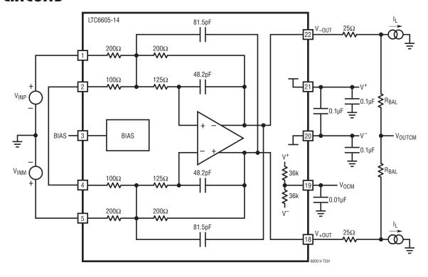
Figure 1. DC Test Circuit (Channel A Shown)
