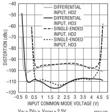
$V_{IN} = 2V_{P-P}, V_{OCM} = 2.5V$ BIAS = 5V, f = 3MHz  $R_L = 400\Omega$  DIFFERENTIAL, GAIN = 1V/V
