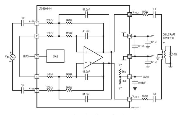
Figure 2. AC Test Circuit (Channel A Shown)
