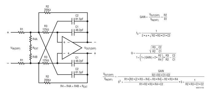
Figure 3. Filter Architecture and Equations
