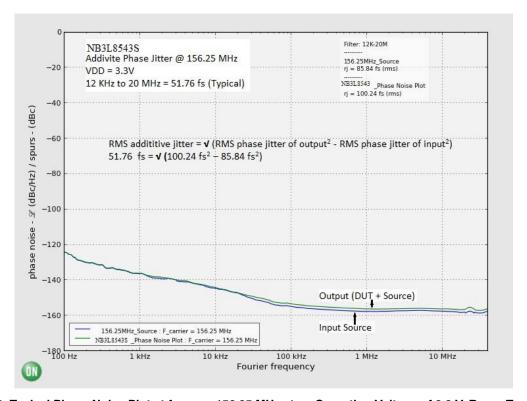
Figure 12. Typical Phase Noise Plot at f<sub>carrier</sub> = 156.25 MHz at an Operating Voltage of 3.3 V, Room Temperature
