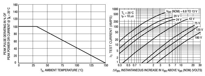
Figure 3. Pulse Derating Curve
