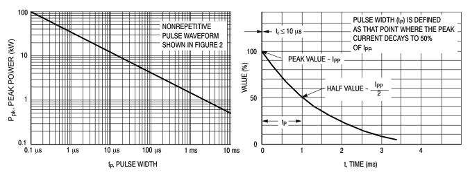
Figure 1. Pulse Rating Curve
