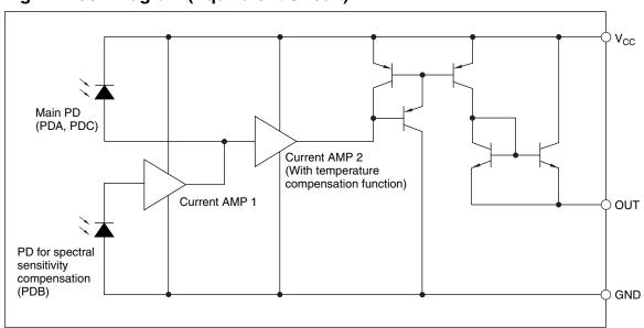
Fig. 2 Block Diagram (Equivalent Circuit)
