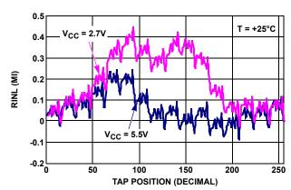
FIGURE 12. RINL vs TAP POSITION IN RHEOSTAT MODE FOR 50k $\Omega$  (U)
