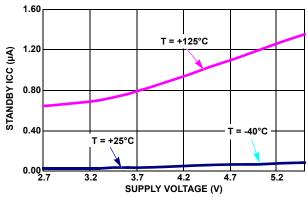
FIGURE 2. STANDBY ICC vs VCC
