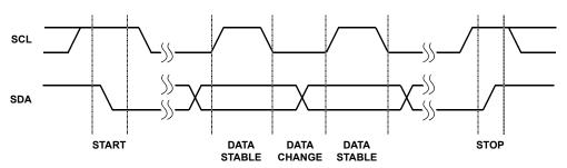
FIGURE 17. VALID DATA CHANGES, START, AND STOP CONDITIONS
