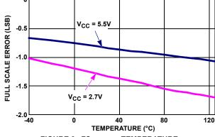
FIGURE 8. FSerror vs TEMPERATURE
