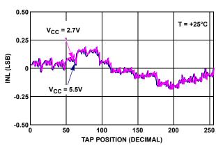
FIGURE 10. INL vs TAP POSITION IN RHEOSTAT MODE FOR 50k $\Omega$  (U)
