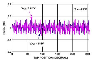
FIGURE 11. RDNL vs TAP POSITION IN RHEOSTAT MODE FOR 50k $\Omega$  (U)
