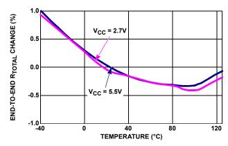
FIGURE 16. END-TO-END R<sub>TOTAL</sub> % CHANGE vs TEMPERATURE, 50k (U)
