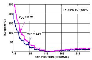
FIGURE 14. TCv FOR VOLTAGE DIVIDER MODE 10k (W) IN  $$\operatorname{ppm}$$
