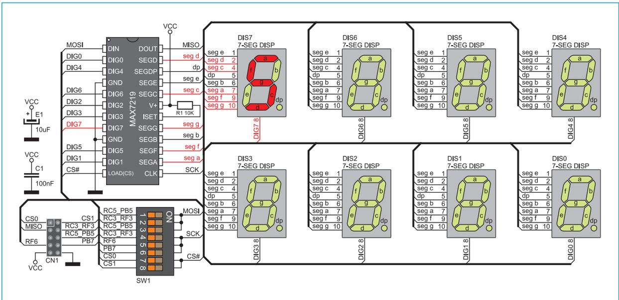
Figure 4: Time-division multiplexing performed on the DIS7 display
