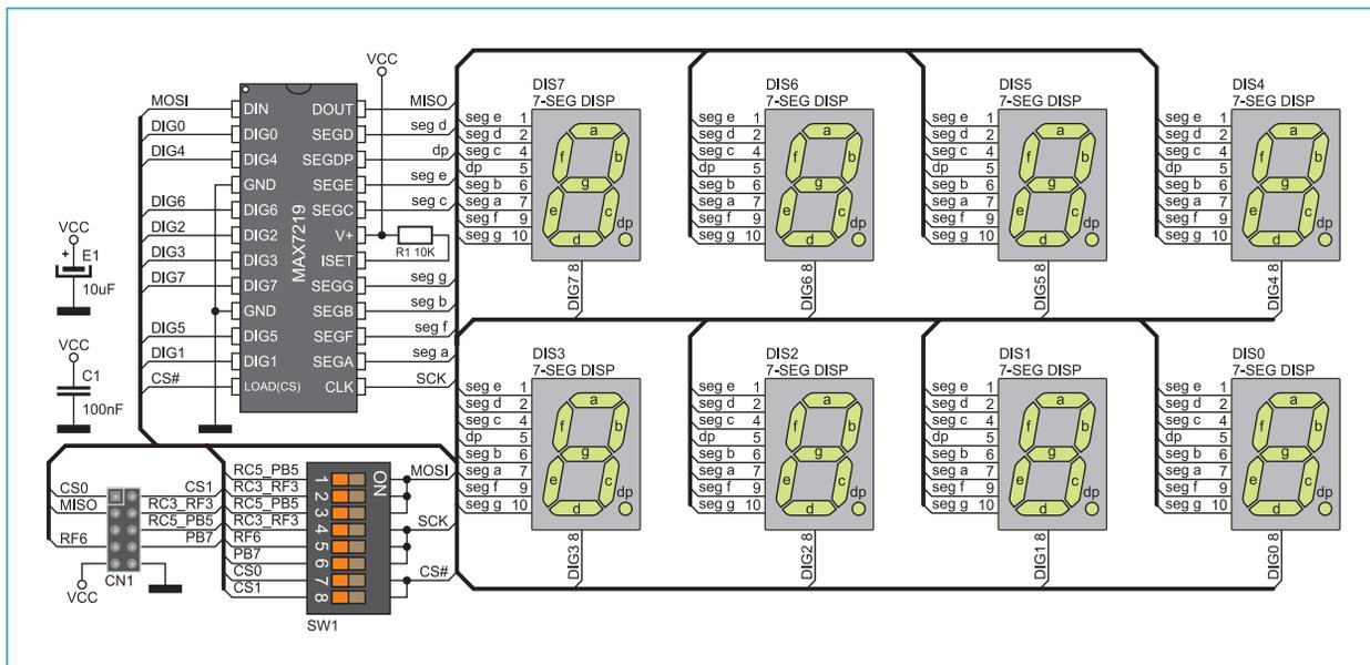
Figure 2: Serial 7-Seg Display 8-Digit additional board connection schematic
