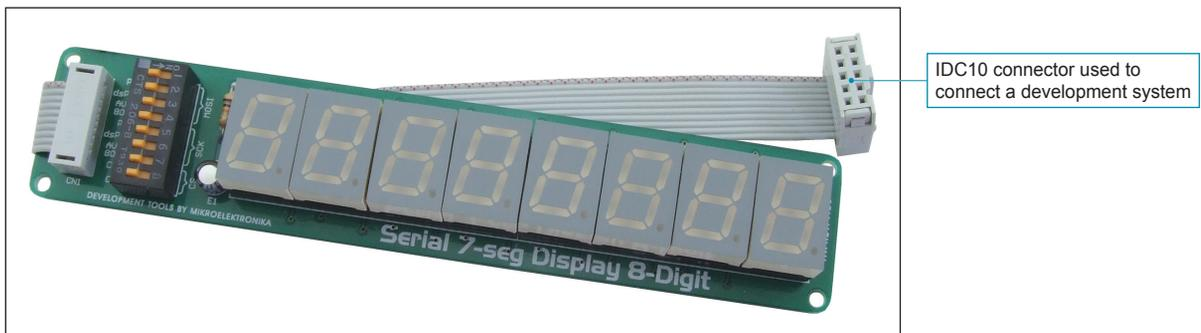
Figure 1: *Serial 7-Seg Display 8-Digit* additional board
