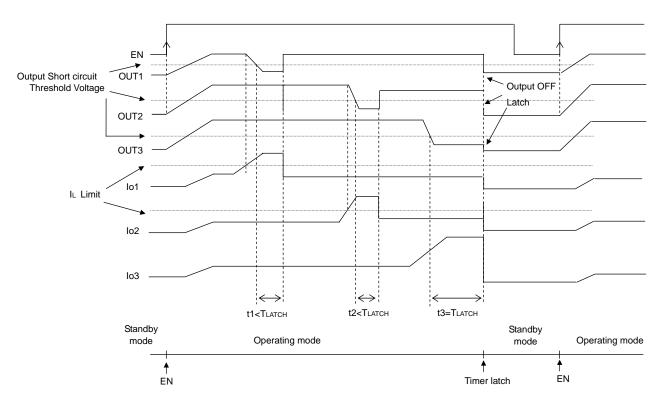
Fig.33 Short-current protection circuit with time delay timing chart
