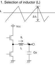
Fig.35 Output ripple current
