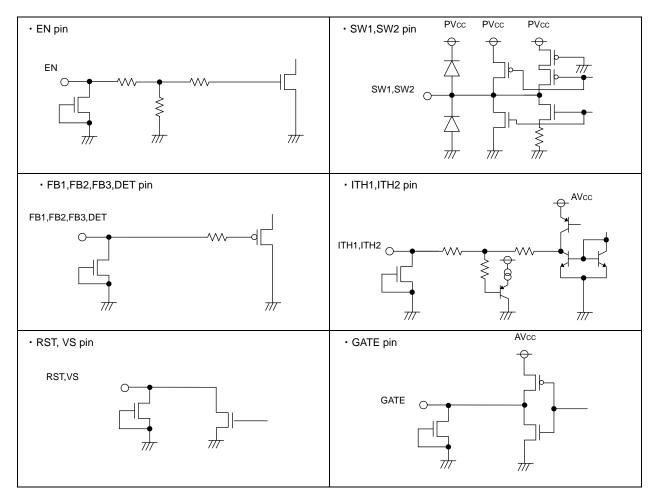
Fig.43 I/O equivalence circuit
