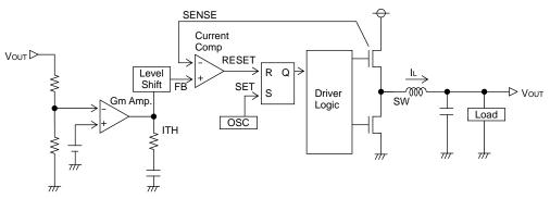
Fig.29 Diagram of current mode PWM control
