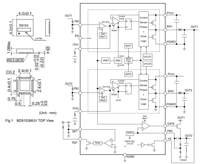
Fig.2 BD9153MUV Block Diagram
