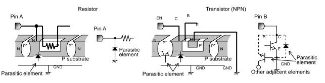
Fig.44 Simplified structure of monorisic IC
