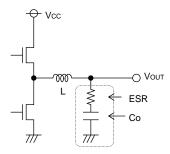
Fig.36 Output capacitor
