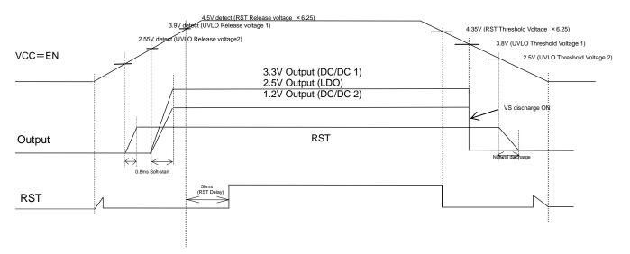
Fig.32 Soft-start, Shutdown, RST Delay, UVLO, timing chart
