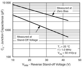
Fig. 4 - Typical Junction Capacitance
