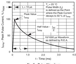
Fig. 3 - Pulse Waveform
