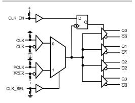
Figure 1. Simplified Logic Diagram of NB3L8533
