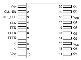
Figure 2. Pinout Diagram (Top View)
