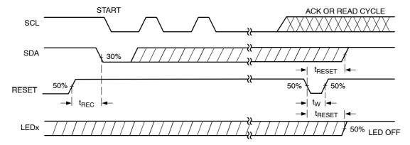
Figure 12. RESET Timing Diagram
