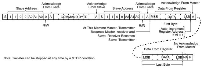
Figure 10. Read from Register Timing Diagram
