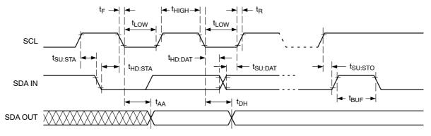
Figure 4. 2-Wire Serial Interface Timing
