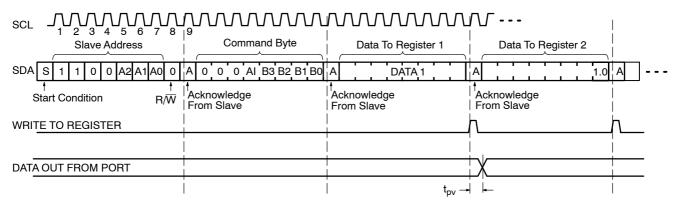
Figure 9. Write to Register Timing Diagram
