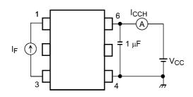
Fig. 12.1.5 I<sub>CCH</sub> Test Circuit
