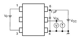
Fig. 12.1.4 V<sub>OL</sub> Test Circuit
