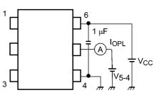
Fig. 12.1.2 I<sub>OPL</sub> Test Circuit
