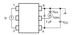
Fig. 12.1.1 I<sub>OPH</sub> Test Circuit
