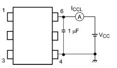
Fig. 12.1.6 I<sub>CCL</sub> Test Circuit
