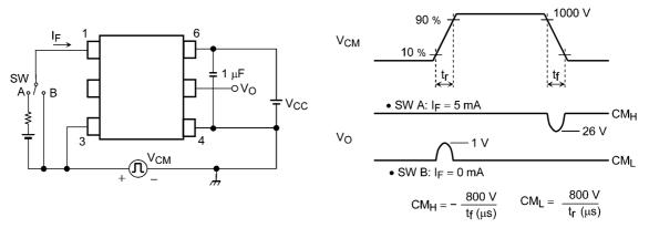
Fig. 12.1.8 Common-Mode Transient Immunity and Waveform
