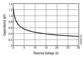
Figure 3. Capacitance vs Reverse Voltage (SMV1430)
