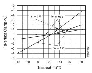
Figure 2. Relative Capacitance Change vs Temperature
