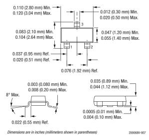
Figure 7. SOT-23 Package Dimensions
