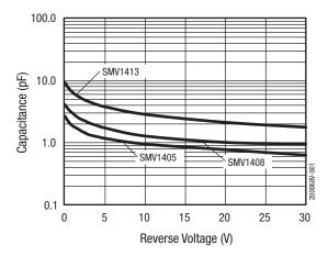
Figure 1. Capacitance vs Reverse Voltage
