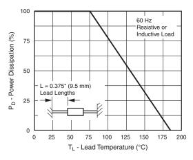
Fig. 5 - Power Derating Curve
