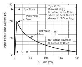
Fig. 3 - Pulse Waveform
