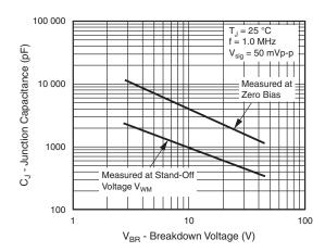
Fig. 4 - Typical Junction Capacitance
