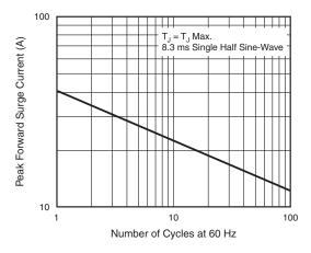
Fig. 6 - Maximum Non-Repetitve Peak Forward Surge Current
