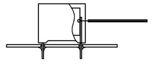
Temperature monitored inside the capacitor.
