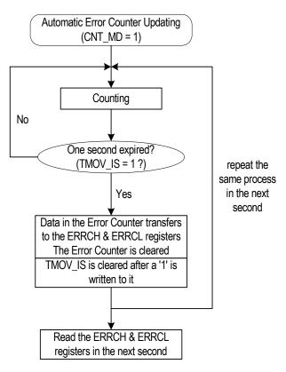
Figure-23 Automatic Error Counter Updating
