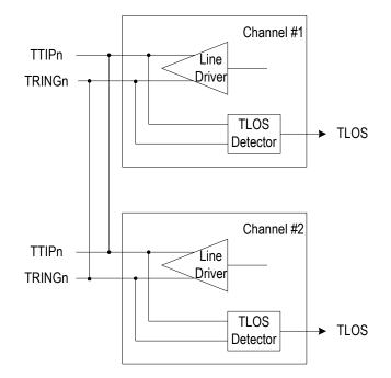
Figure-18 TLOS Detection Between Two Channels
