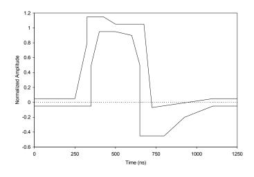
Figure-9 DSX-1 Waveform Template
