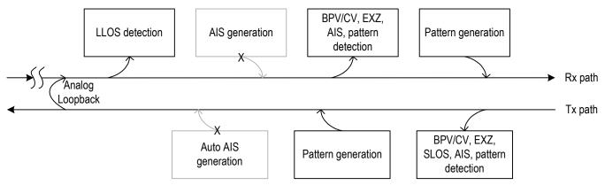
Figure-25 Priority Of Diagnostic Facilities During Analog Loopback
