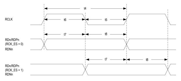
Figure-39 Receive Clock Timing Diagram
