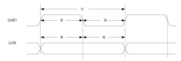
Figure-40 CLKE1 Clock Timing Diagram
