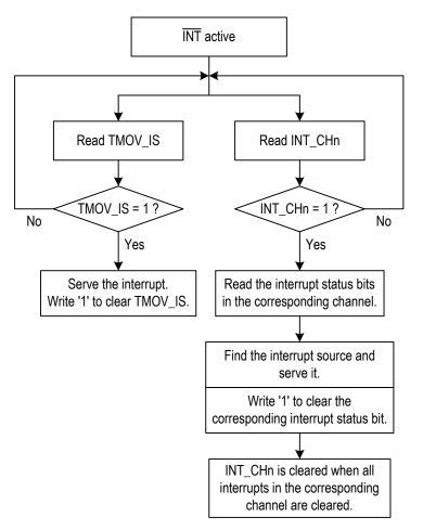
Figure-31 Interrupt Service Process
