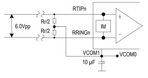
Note: 1. Two Rr/2 resistors should be connected to VCOM[1:0] that are coupled to ground via a 10  $\mu$ F capacitor, which provide 60  $\Omega$ common mode input resistance.
