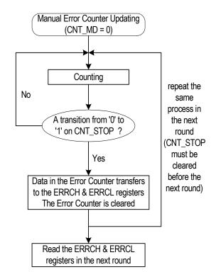
Figure-24 Manual Error Counter Updating
