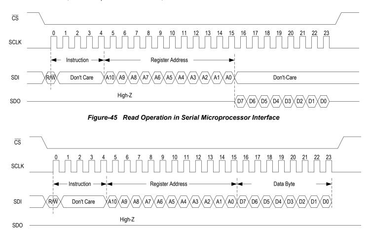
Figure-46 Write Operation in Serial Microprocessor Interface
