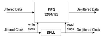
Figure-16 Jitter Attenuator
