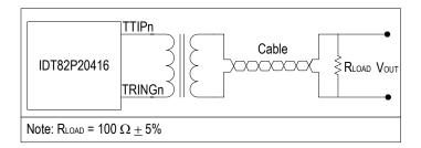
Figure-10 T1 Waveform Template Measurement Circuit
