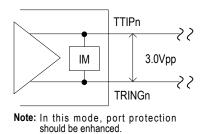
Figure-15 Transmit Differential Line Interface with Twisted Pair Cable (transformer-less, non standard compliant)
