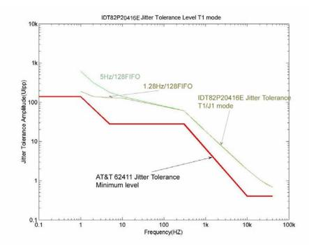
Figure-42 T1/J1 Jitter Tolerance Performance
