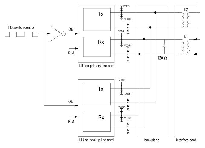
**Rx:** Partially Internal Impedance Matching mode. A fixed external 120  $\Omega$  resistor is placed on the backplane and provides a common termination for T1/J1/E1 applications. The R\_TERM[2:0] bits (b2~0, RCF0,...) setting is as follows: '000' for T1 100  $\Omega$  twisted pair cable, '001' for J1 110  $\Omega$  twisted pair cable, '010' for E1 120  $\Omega$  twisted pair cable and '011' for E1 75  $\Omega$  coaxial cable.
