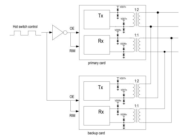
**Rx:** Fully Internal Impedance Matching mode. In this mode, there is no external resistor required. The R\_TERM[2:0] bits (b2~0, RCF0,...) setting is as follows: '000' for T1 100 $\Omega$  twisted pair cable, '001' for J1 110  $\Omega$  twisted pair cable, '010' for E1 120  $\Omega$  twisted pair cable and '011' for E1 75  $\Omega$  coaxial cable.
