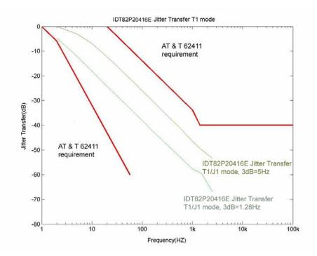
Figure-44 T1/J1 Jitter Transfer Performance
