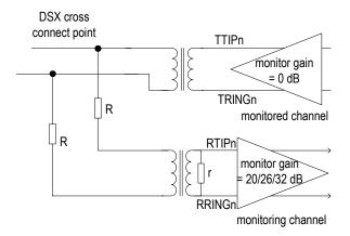
Figure-8 Transmit Path Monitoring
