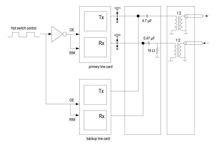
**Rx:** 75  $\Omega$  External Impedance Matching mode. In this mode, there is no external resistor required. The RIM pin should be left open and the configuration of the R\_TERM[2:0] bits (b2~0, RCF0,...) is ignored.
