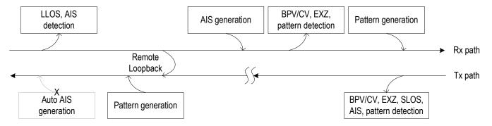
Figure-26 Priority Of Diagnostic Facilities During Manual Remote Loopback
