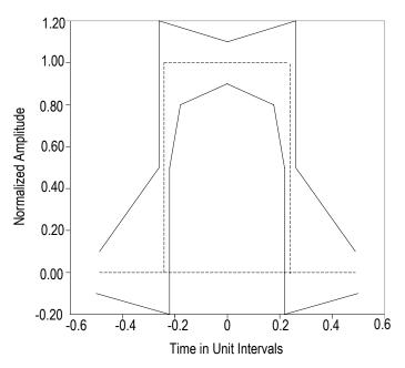
Figure-11 E1 Waveform Template
