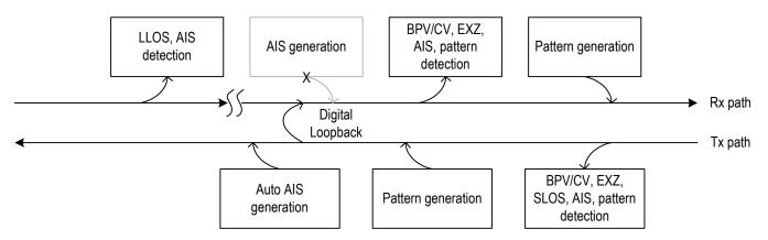
Figure-27 Priority Of Diagnostic Facilities During Digital Loopback
