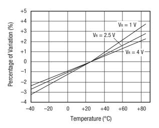
Figure 2. Relative Capacitance Change vs Temperature
