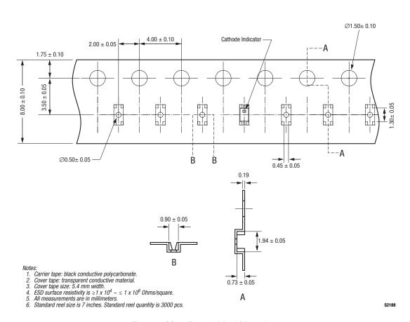
**Figure 7. SC-79 Tape and Reel Dimensions**
