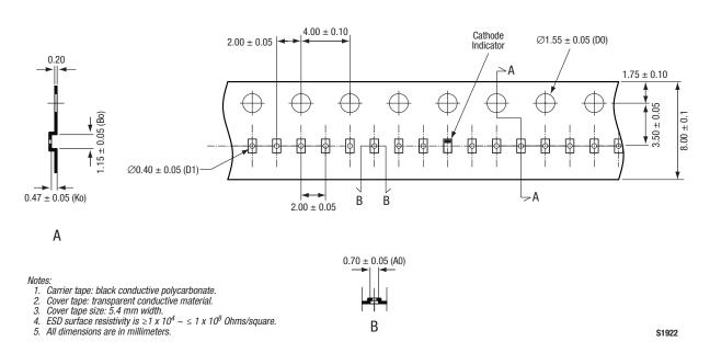
Figure 9. SOD-882 Tape and Reel Dimensions
