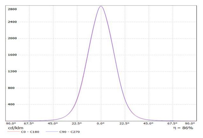
Luminaire: Ledil Oy FA11941\_LXM\_REC FA11941\_LXM\_REC LOR=82% Lamps: 1 x Cree XM-L
