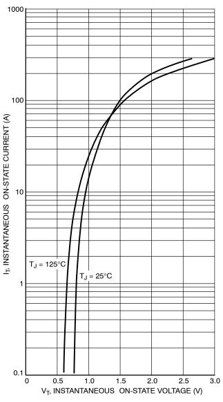
Figure 3. On-State Typical Characteristics
