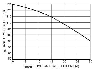
Figure 1. RMS Current Derating
