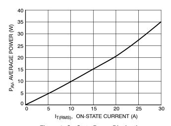
Figure 2. On-State Power Dissipation
