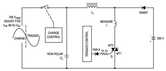
Note: Component values are for verification of rated (di/dt)<sub>c</sub>. See AN1048 for additional information.
