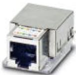
RJ45 socket insert, for the Freenet system, CAT6, 8-pos., shielded, with cable connection (IDC fast connection), for litz and solid wires AWG 24 ... 22
