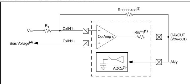
$$V_{OAxOUT} = \left(\frac{R_{FEEDBACK}}{R_1}\right) (Bias\ Voltage - V_{IN})$$
