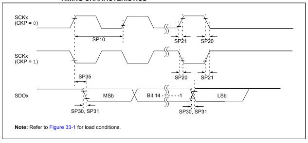
FIGURE 33-16: SPI2 AND SPI3 MASTER MODE (HALF-DUPLEX, TRANSMIT ONLY, CKE = 1) TIMING CHARACTERISTICS
