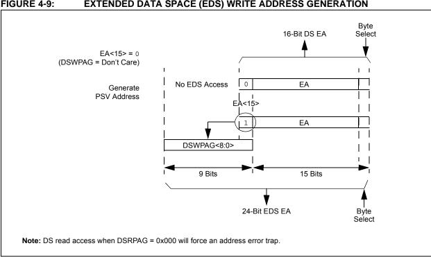
FIGURE 4-9: **EXTENDED DATA SPACE (EDS) WRITE ADDRESS GENERATION**
