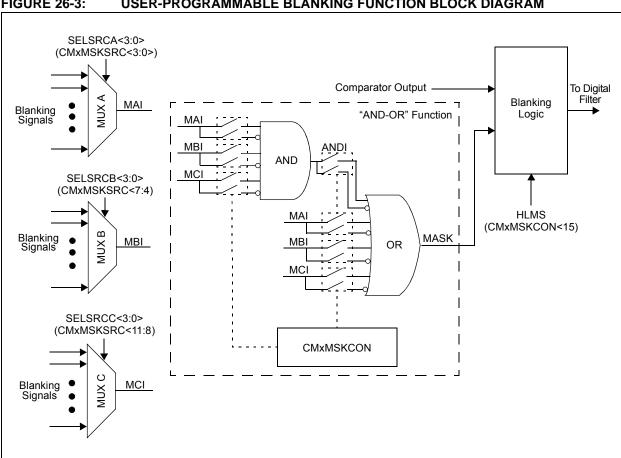
**FIGURE 26-3:** USER-PROGRAMMABLE BLANKING FUNCTION BLOCK DIAGRAM
