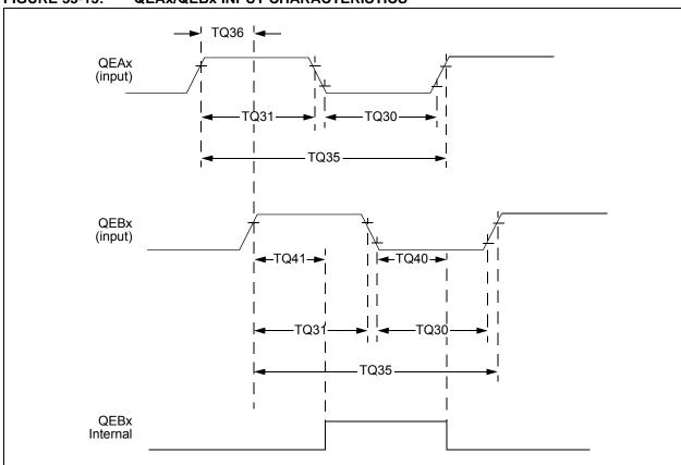
FIGURE 33-13: QEAX/QEBX INPUT CHARACTERISTICS
