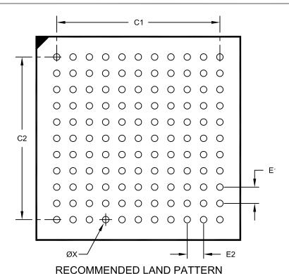
Units **MILLIMETERS Dimension Limits** MIN MOM MAX Contact Pitch E1 0.80 BSC Contact Pitch E2 0.80 BSC Contact Pad Spacing 8.00 C1 Contact Pad Spacing 8.00 C2 Contact Pad Diameter (X121) Χ 0.32
