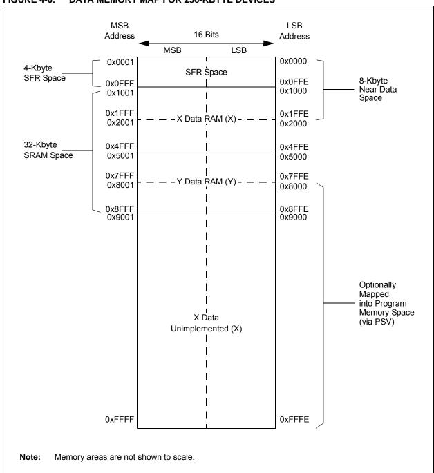
FIGURE 4-6: DATA MEMORY MAP FOR 256-KBYTE DEVICES
