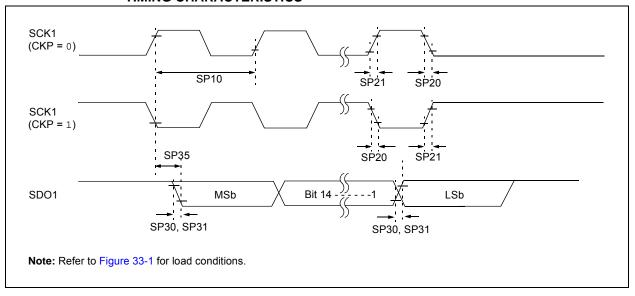
FIGURE 33-24: SPI1 MASTER MODE (HALF-DUPLEX, TRANSMIT ONLY, CKE = 1) TIMING CHARACTERISTICS
