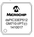
100-Lead TQFP (14x14x1 mm)
