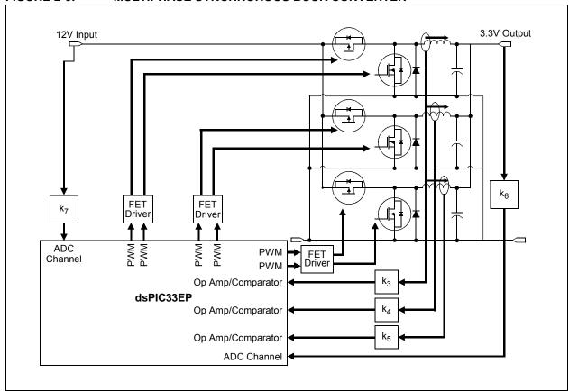
FIGURE 2-7: INTERLEAVED PFC
