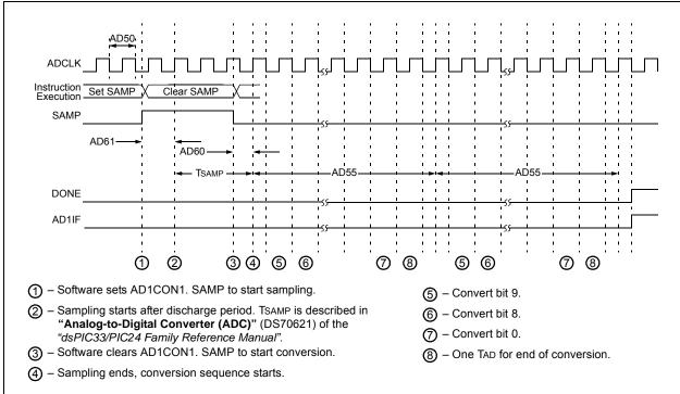
FIGURE 33-40: ADC1 CONVERSION (10-BIT MODE) TIMING CHARACTERISTICS (CHPS<1:0> = 01, SIMSAM = 0, ASAM = 1, SSRC<2:0> = 111, SSRCG = 0, SAMC<4:0> = 00010)
