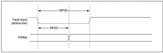
FIGURE 33-11: HIGH-SPEED PWMx MODULE TIMING CHARACTERISTICS
