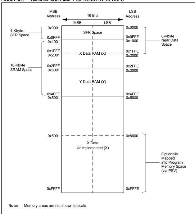
FIGURE 4-5: DATA MEMORY MAP FOR 128-KBYTE DEVICES
