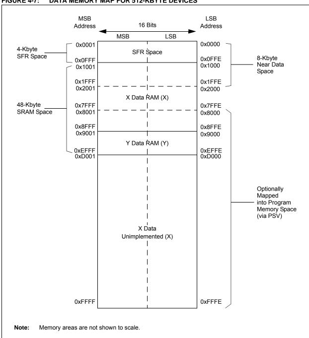
FIGURE 4-7: **DATA MEMORY MAP FOR 512-KBYTE DEVICES**
