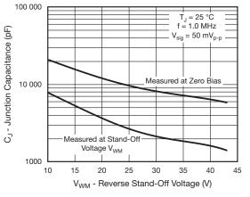
Fig. 6 - Typical Junction Capacitance
