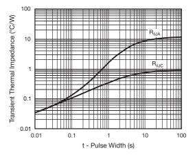
Fig. 5 - Typical Transient Thermal Impedance
