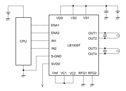
Constant voltage control mode: OUT outputs a 1.75 V, which is Vref (0.9 V)  $\times$  1.95.  $\ast$  : FC1 and FC2 are left open.
